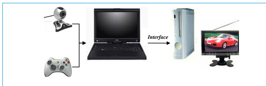
Figure 3. Hardware setup of the vision-based HMI for Xbox [1].
