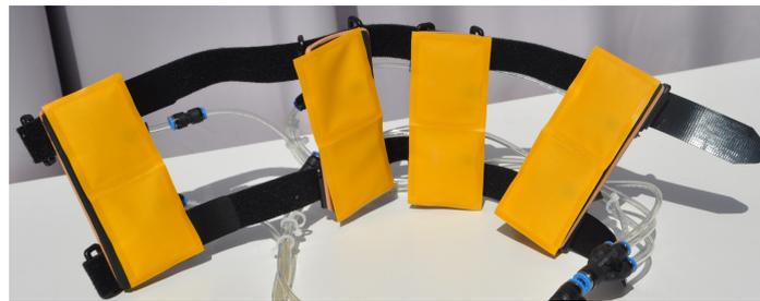
**Figure 3.** First prototype of sensor system using pneumatic padding for the upper arm based on eight air-pads that are manufactured by the company Dr. Winkler GmbH & Co. KG (Ainring, Germany).
