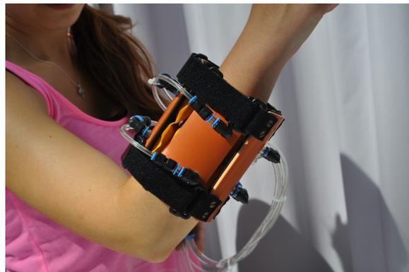
**Figure 1.** First prototype of human-robot interface for wearable robotic device with integrated pneumatic padding. Using pressure sensors and artificial neural networks (ANNs) the interaction forces/torques between a user and robot can be roughly estimated.
