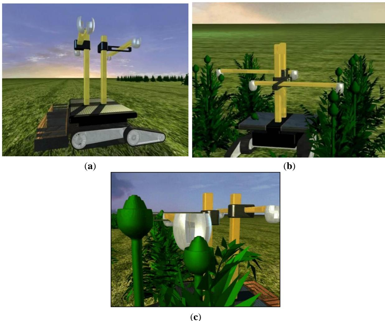
The control architecture should be composed by four main blocks: the vision system, the mobile platform position control system, the manipulators control system and the main supervising and coordinating control system. Once the supervising and coordinating block is signaled from the vision system that an artichoke is found in the image in a suitable workspace, it stops the mobile base at the
