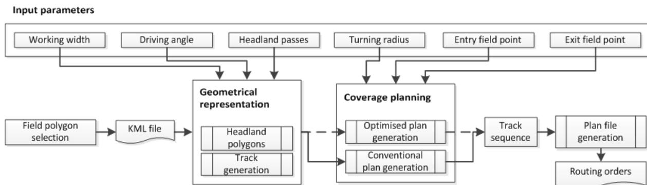
The final function is the generation of the routing orders, which include a sequence of straight lines and turnings executions. Straight line segments are described by the heading, the distance to be travelled, the driving speed and the starting X and Y coordinates. Turning segments are described by the initial heading, the final heading, the direction of the turn (clockwise or anti-clockwise) and the driving speed.
