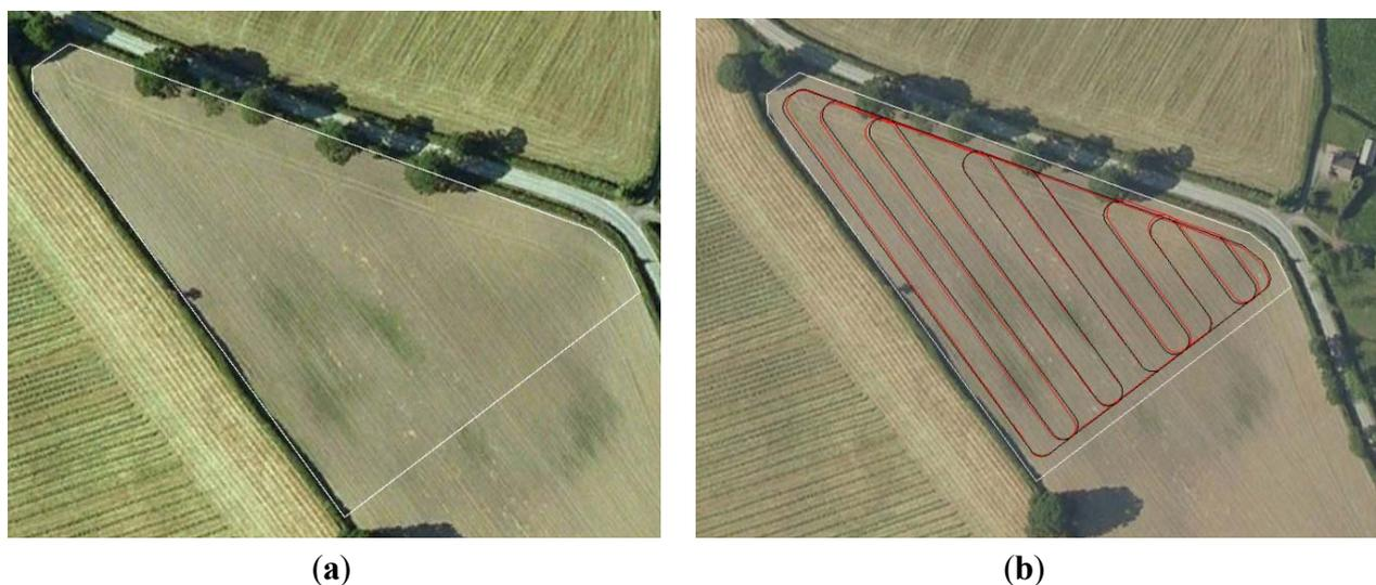
The field used is located at 52.42° N, 2.58° W, and the dimensions were sampled from Google Earth and scaled down by 1:14 to be relative to the test platform. The route was planned using a working width of 0.714 m (approximately, in full scale, 10 m) and driving parallel to the longest edge of the field.
