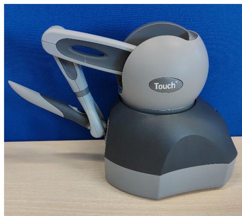
**Figure 2.** The Geomagic Touch haptic interface.
