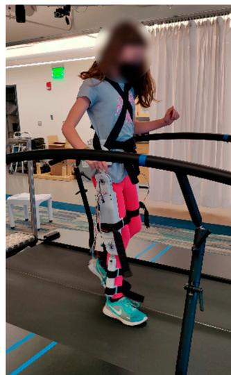
**Figure 4.** Pediatric participant walking on the instrumented treadmill while wearing the adjustable pediatric exoskeleton.
