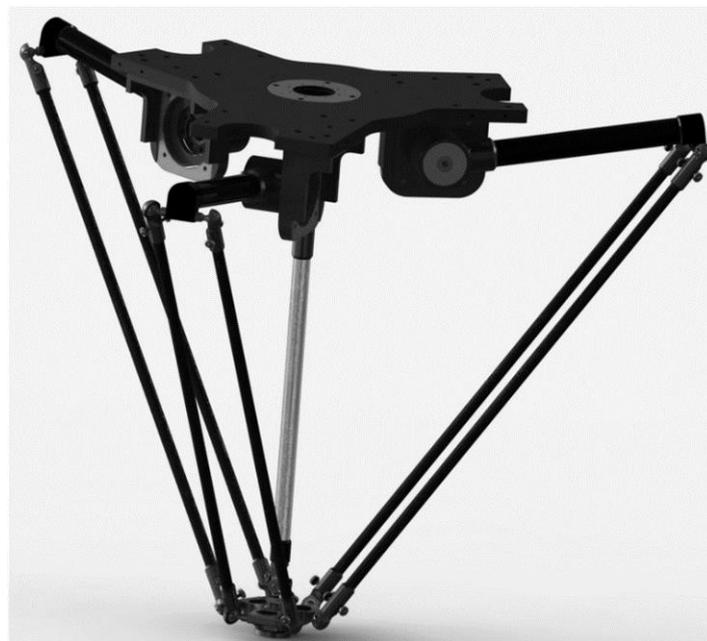
**Figure 1.** The mechanical structure of the Delta robot with telescopic rod.
