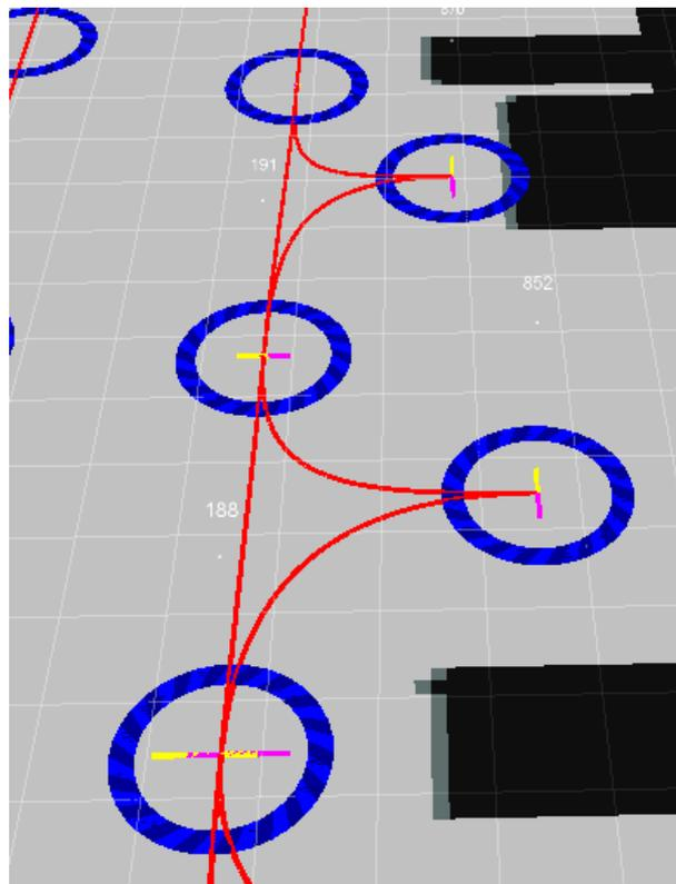
Figure 2. Cubic Bézier Curves Example.
