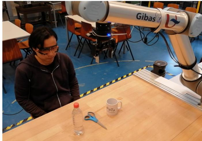
**Figure 1.** The scenario where a human can select one of the objects on the table using eye-tracking glasses and a robotic manipulator will pick up the selected object.
