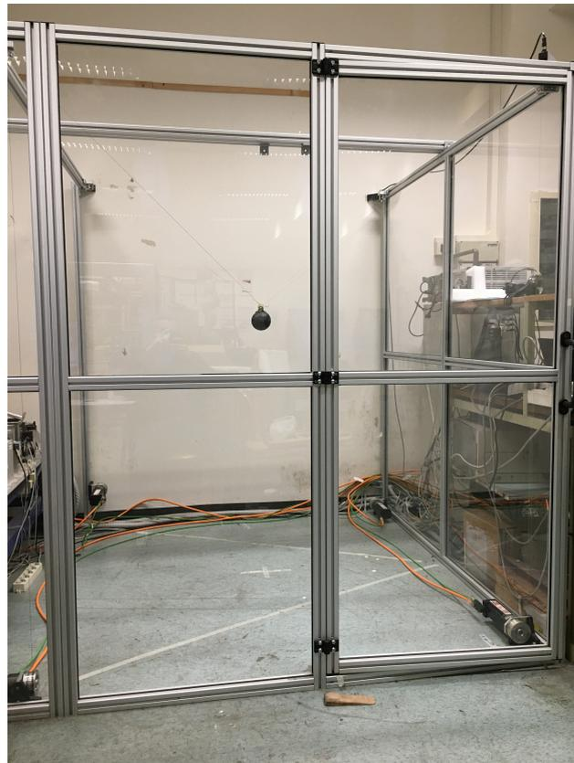
**Figure 5.** Prototype cable suspended parallel robot (CSPR) used during the tests.
