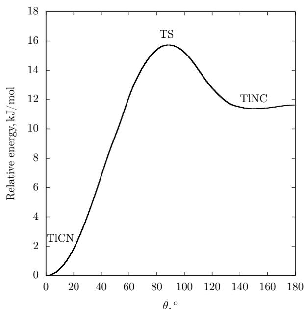
**Figure 2.** The cross section of RCCSD(T)/CBS potential energy surface for TI·CN along the approximate isomerization path. TS: transition state. The energy is given with respect to the global minimum. The distance  $r(\text{CN}) = 1.16641 \text{ \AA}$  is frozen at the equilibrium value for the TICN isomer.
