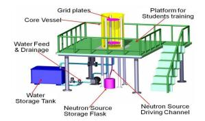
Figure 1. Schematic design of the subcritical reactor systems and platform [4].
