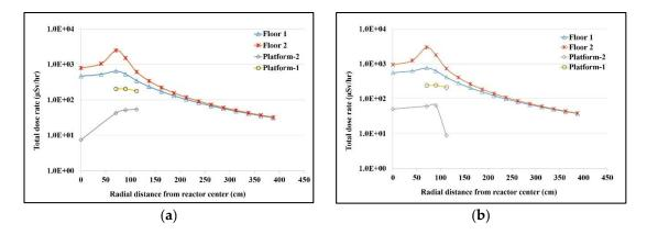
**Figure 6.** The total dose rate in the reactor hall during start-up and shut-down operations: (**a**) Using ICRP-74 flux-to-dose conversion factors; (**b**) Using ANSI/ANS flux-to-dose conversion factors.
