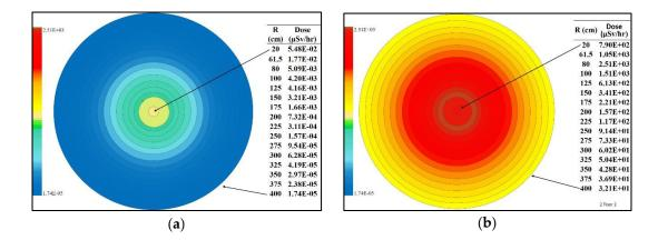
**Figure 7.** Spectrum of the dose rate ( $\mu$ Sv/hr) vs. the radial distance from the reactor centerline, for cells number 40 through 55 at the floor 2 level (120–170 cm in height) using ICRP-74 factors: (**a**) During normal operation mode; (**b**) During start-up/shut-down operation mode.
