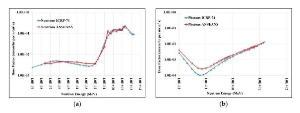
**Figure 2.** The flux-to-dose equivalent rate conversion factors on a log-log scale, as recommended by the ICRP and ANSI: (a) Neutrons (b) Photons.
