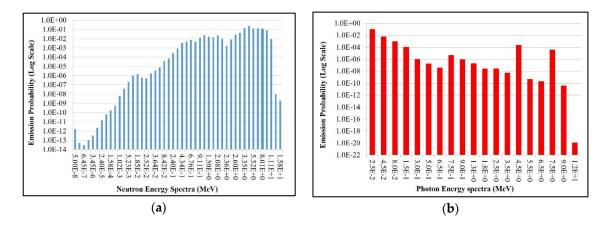
**Figure 3.** MCNP modeling of the probability distribution of the source neutrons and photons emissions: (a) Using 47 energy bins for neutrons; (b) Using 19 energy bins for photons.
