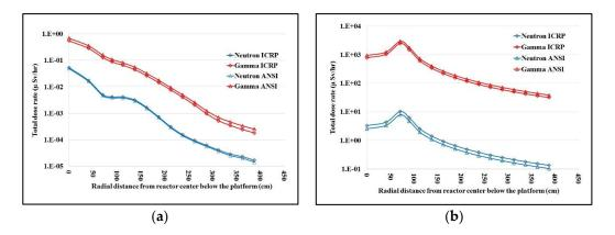
**Figure 8.** The total dose rate ( $\mu$ Sv/hr) from neutrons and gammas, in the reactor hall below the platform level (floor 2), using ICRP-74 and ANSI/ANS factors: (**a**) During normal operation mode; (**b**) During start-up/shut-down operation mode.
