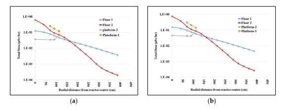
**Figure 5.** The total dose rate in the reactor hall vs. the radial distance from the reactor center during normal operation: (**a**) Using ICRP-74 flux-to-dose conversion factors; (**b**) Using ANSI/ANS flux-to-dose conversion factors.
