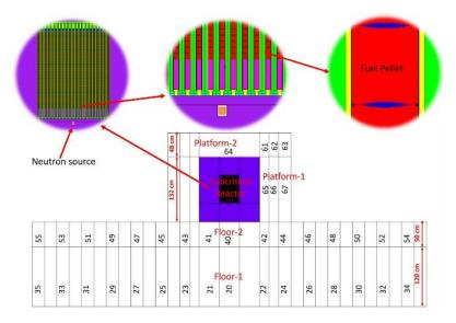
**Figure 4.** MCNP cross-sectional view (x-z) of dose mapping zones in the subcritical reactor hall, showing the height of floor 1, floor 2, platform 1, platform 2 (in red), and the cell numbers (in black). Magnified view of the core with the neutron source, fuel rods, and fuel pelt are shown on top.
