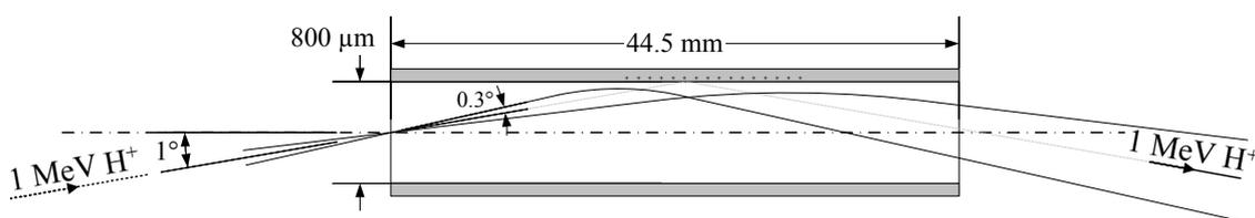
**Figure 1.** Schematic picture of our cylindrical shaped PTFE capillary sample. Note: the X and Y scales are different from the drawing, but the incident angle is shown as per calculations from the distances.
