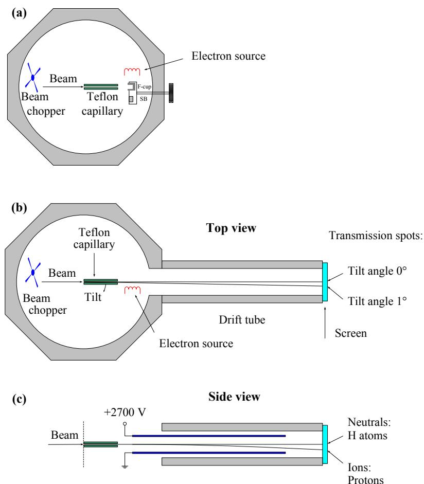
**Figure 2.** (Color online). Schematic view of the experimental setup: (a) was used for transmission measurements (Faraday-cup) and for energy determination (SB-detector); (b) is the top view of the fluorescent screen setup. It shows the observation of the beam spot shift due to the rotation; (c) is the side view. It shows the separation of charged and neutral particles.
