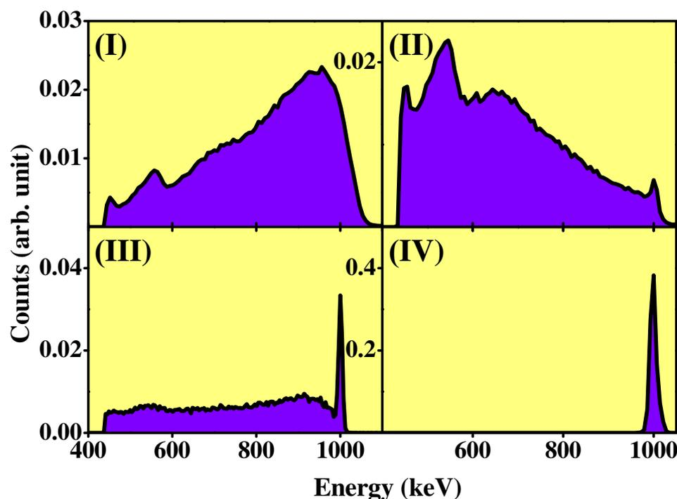
**Figure 4.** (Color online). Evolution of the energy distribution of the transmitted beam according to the time indicating by Roman numbers in figure 3. (I) At the time when the beam just entered to the capillary (the transmission rate was 25 %), (II) at the time when the transmission rate was 40 % (III) at the time when the transmission rate was 60 %, and (IV) at the time when stable transmission was achieved.
