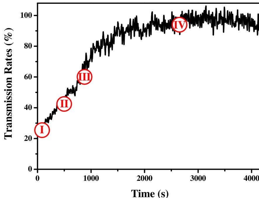
**Figure 3.** (Color online). Time dependence of the transmission rates. After the charge-up process the guiding remained stable until the measurement was stopped. The charge accumulated on the capillary wall was less than 14 nC, the surface charge density was  $12 \text{ nC/mm}^2$ . Circles with Roman numbers inside show the spectrum analysis moments.
