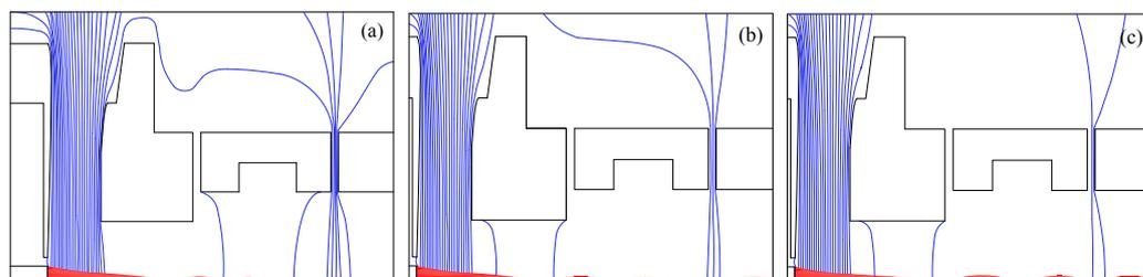
**Figure 2.** Simulated trajectories (red) and equipotential lines (blue) for an electron beam with an energy  $E$  of: (a) 11.5 keV; (b) 15 keV; (c) 25 keV. Electron current  $I = 20$  mA in all cases. Part of the drift tube section with an enlarged diameter corresponds to the area under radiation control.
