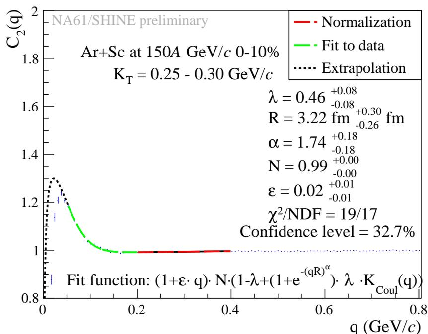
**Figure 2.** Example fit with Bose–Einstein correlation function at  $K_T = 0.25\text{--}0.30$  GeV/c for the sum  $(\pi^+ + \pi^+) + (\pi^- + \pi^-)$ . Blue points with error bars represent the data, the green dash-dotted line
