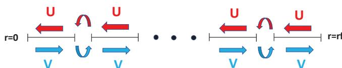
**Figure 4.** Sketch of the application of the boundary conditions between the different subdomain grids. Through an analysis of the characteristics, the flow of the field variables  $u$  and  $v$  can be identified (in our case  $u$  and  $v$  would correspond to  $\rho, M, R, U$ ), and we apply the prescription of Equation (72).
