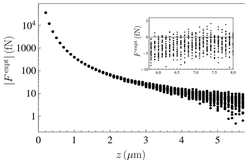
**Figure 3.** All measured magnitudes of the Casimir force between an Au-coated sphere and an Au-coated plate obtained from the first harmonic of the interaction as the plate rotates under the sphere are shown as a function of separation (in a logarithmic scale). The inset shows the force values over the region of large separations (in a linear scale).
