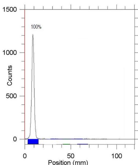
**Fig. 2.** ITLC of [<sup>67</sup>Ga]GaCl<sub>3</sub> in pure methanol as mobile phase on Whatman No.2 papers.
