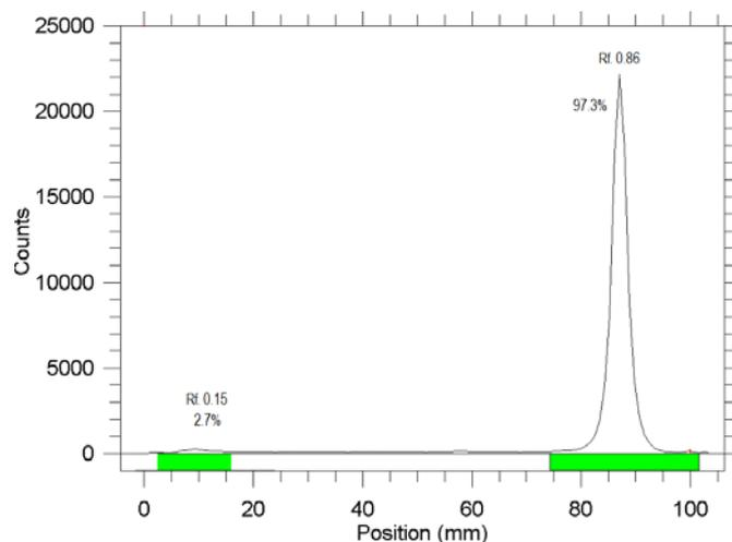
**Fig. 3.** ITLC of  $[^{67}\text{Ga}][\text{APTSM}_2]_2^+$  in pure methanol as mobile phase on Whatman No.2 papers.
