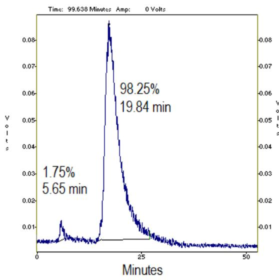
**Fig. 4.** HPLC chromatogram of  $[^{67}\text{Ga}][\text{APTSM}_2]_2^+$  solution on a reversed phase column using acetonitrile + 0.1% TFA/water + 0.1% TFA, 90:10
