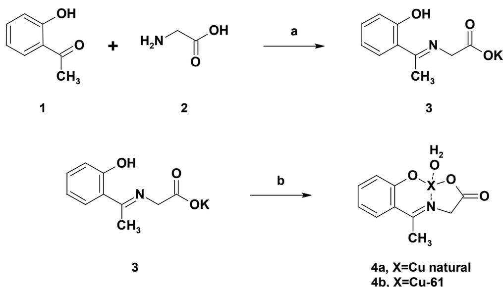
**Fig. 1.** Synthesis of precursor, K<sup>+</sup>NHAG **3**, and Cu-NHAG **4a,b**;
