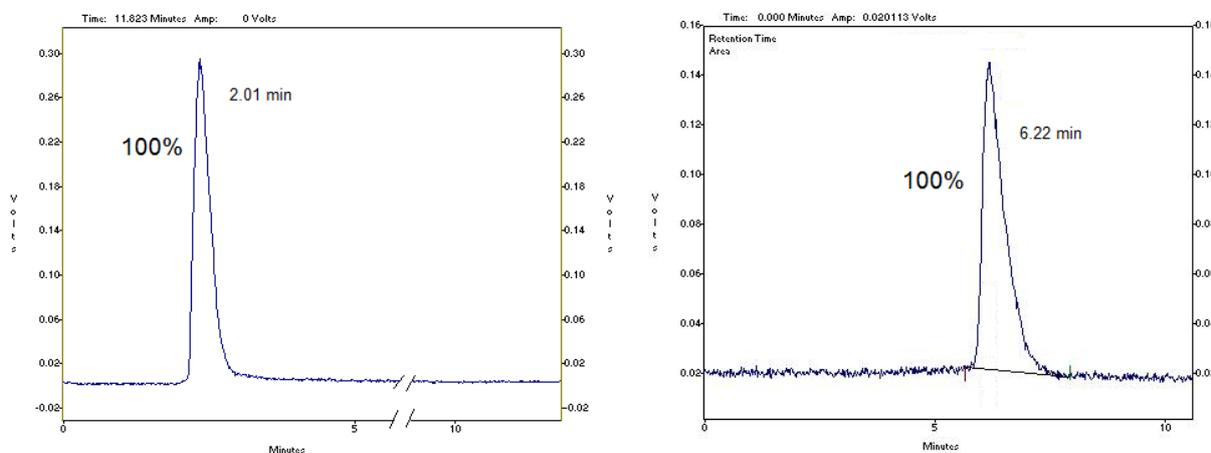
**Fig. 4.** HPLC diagram for [ $^{61}\text{Cu}$ ]Cu<sup>2+</sup> (in acetate and chloride form, left) and [ $^{61}\text{Cu}$ ]NHAG (right) using a reverse phase column with a mixture of H<sub>2</sub>O:CH<sub>3</sub>CN (1:1) as eluent
