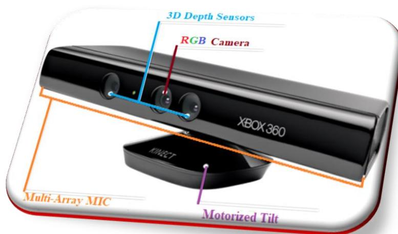
**Figure 29.** Microsoft Kinect Sensor.
