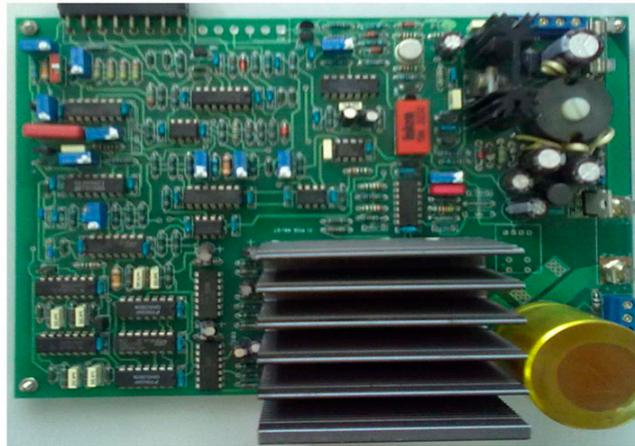
Figure 4. DC motor driver (60 V,  $\pm 10$  A) [21].
