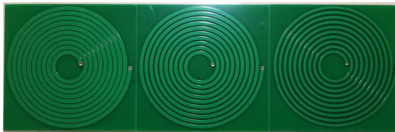
Figure 20. Group-3 prototypes with track width 5 mm (left), 4 mm (middle) and 3 mm (right).
