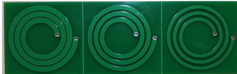
Figure 14. Group-1 prototypes with track width 5 mm (left), 4 mm (middle) and 3 mm (right).
