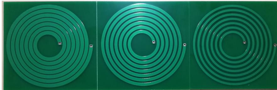
Figure 17. Group-2 prototypes with track width 5 mm (left), 4.2 mm (middle) and 3 mm (right).
