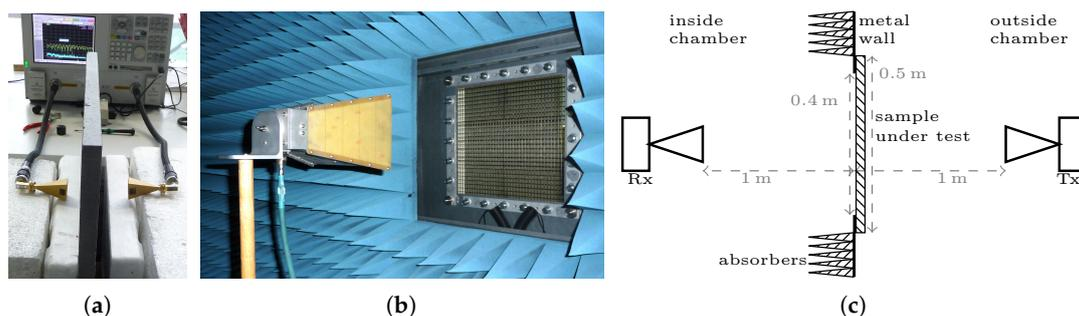
**Figure 3.** Measurement setup. (a) Free space; (b) Anechoic chamber; (c) Schematic of the anechoic chamber setup, with distances.
