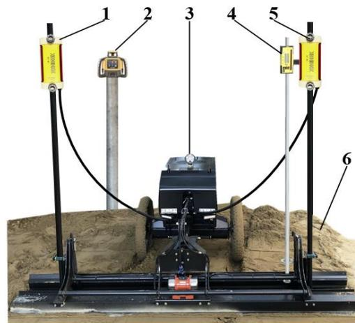
**Figure 12.** Test site of concrete levelling. (1. Left laser receiver, 2. Laser transmitter, 3. Concrete leveler, 4. Level sensor, 5. Right laser receiver, and 6. Sand bed).
