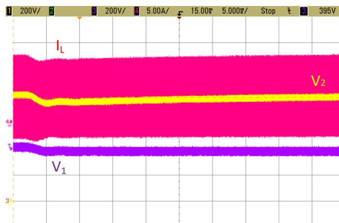
**Figure 14.** Dynamic behavior of the PI regulator over a step in the input voltage.  $V_1$  changes from 400 V to 350 V, keeping  $V_2 = 800$  V.  $V_1$  (violet),  $I_L$  (pink) and  $V_2$  (yellow).
