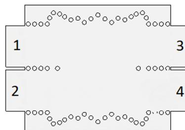
Figure 1. Substrate integrated waveguide 3 dB coupler.
