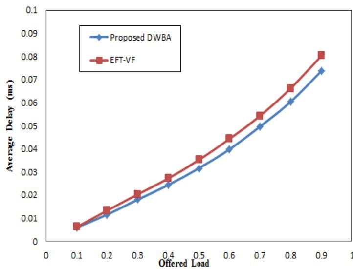
Figure 9. Average packet delay comparison between EFT void filling (VF) and our proposed DWBA at a 10-Gbps data rate per channel.
