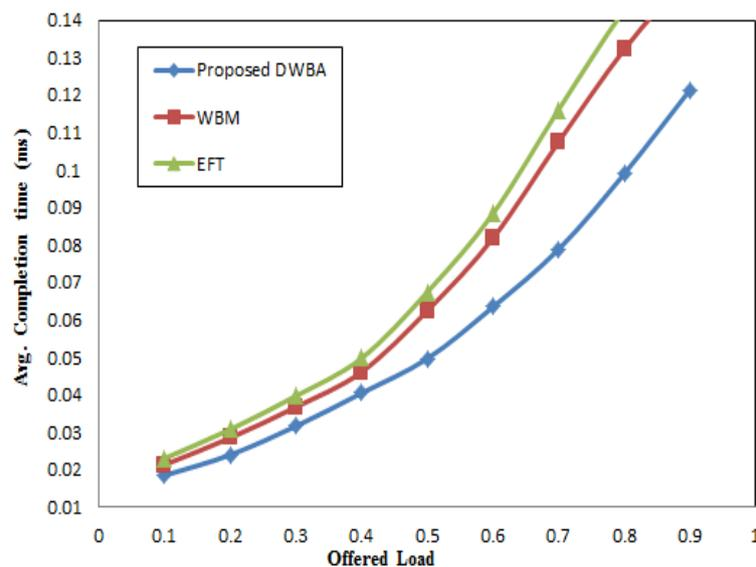
Figure 8. Average completion time of different DWBA algorithms with a 10-Gbps data rate for each channel.
