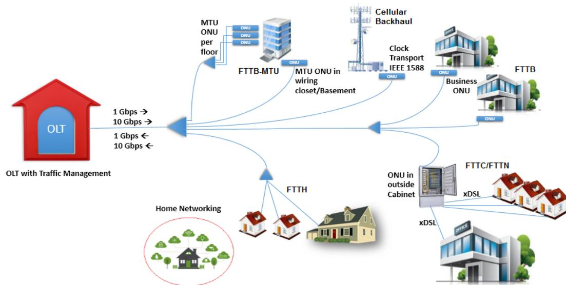
**Figure 1.** Next-generation EPON. ONU, optical network unit; OLT, optical line terminal.
