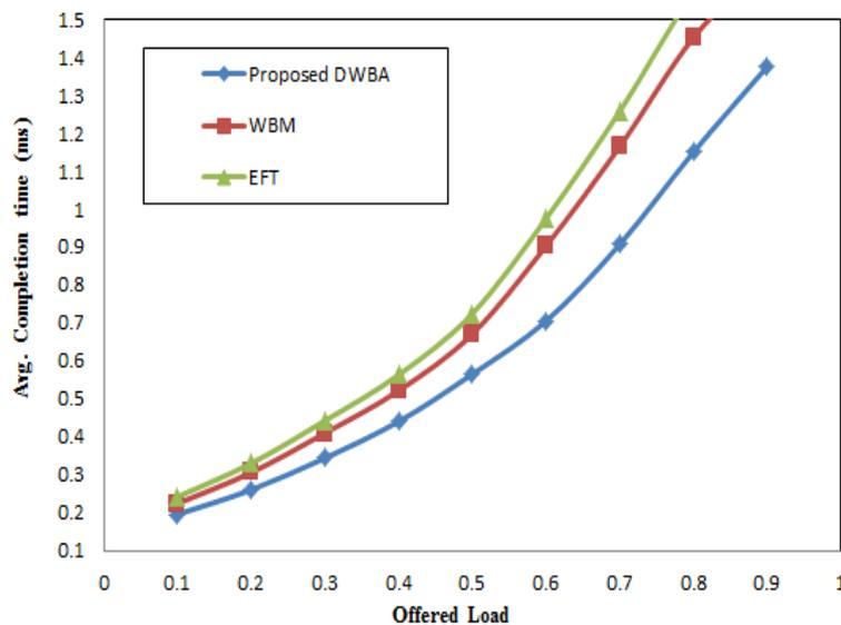
Figure 6. Average completion time of different DWBA algorithms with a 1-Gbps data rate for each channel.
