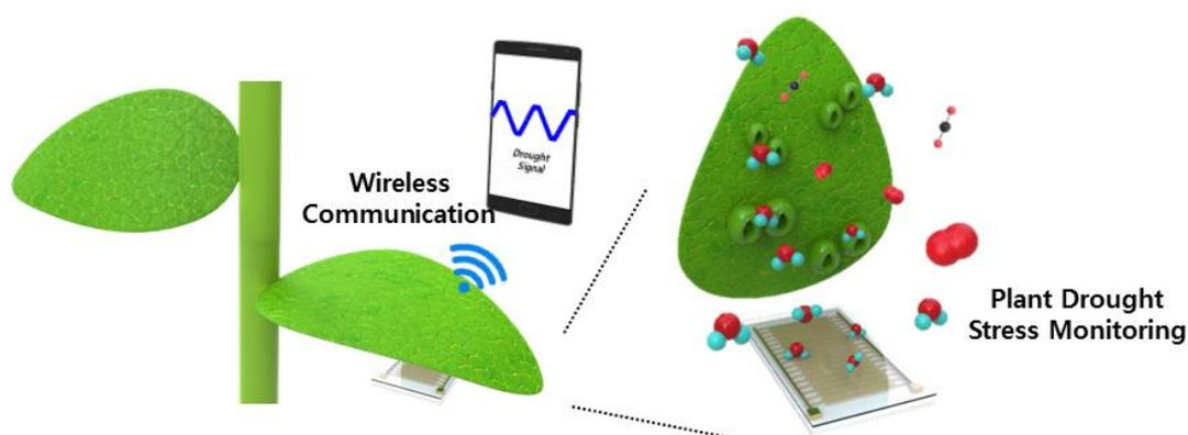
**Figure 1.** Scheme of the flexible PI-based plant drought stress monitoring system.
