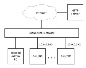
Figure 1. Testbed setup.
