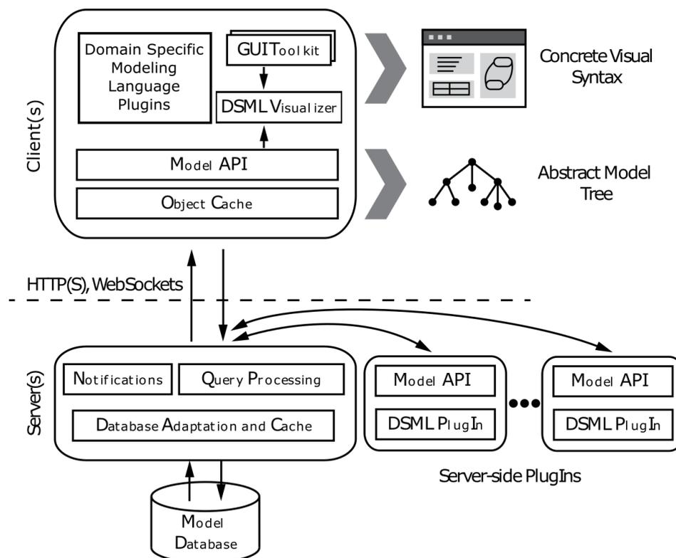
**Figure 8.** Architectural overview of WebGME and its server, browser, client, plugin, and visualization systems.
