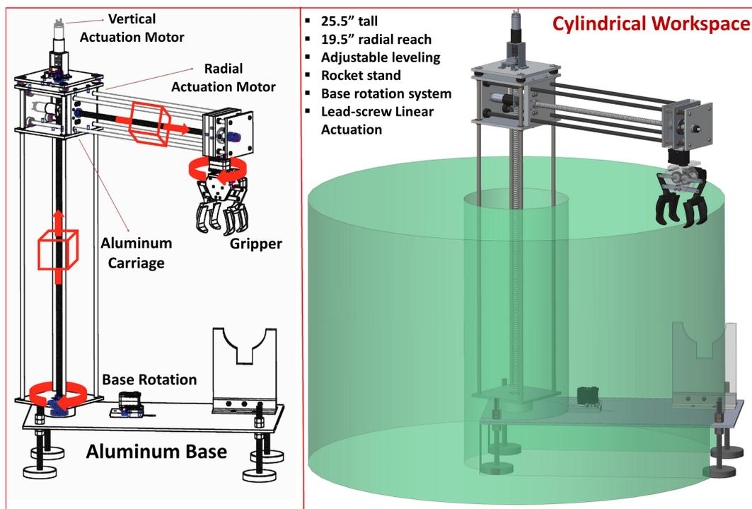
Figure 23. AGSE Mechanical Design.
