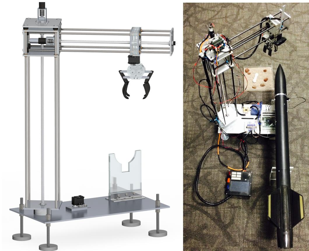
**Figure 18.** AGSE and rocket used in the 2014–2015 NASA SLI competition. The UIP is shown in the bottom left of the picture, the Motor Control Board is on the top of the arm of the AGSE, and the NVIDIA Jetson is under the rocket.
