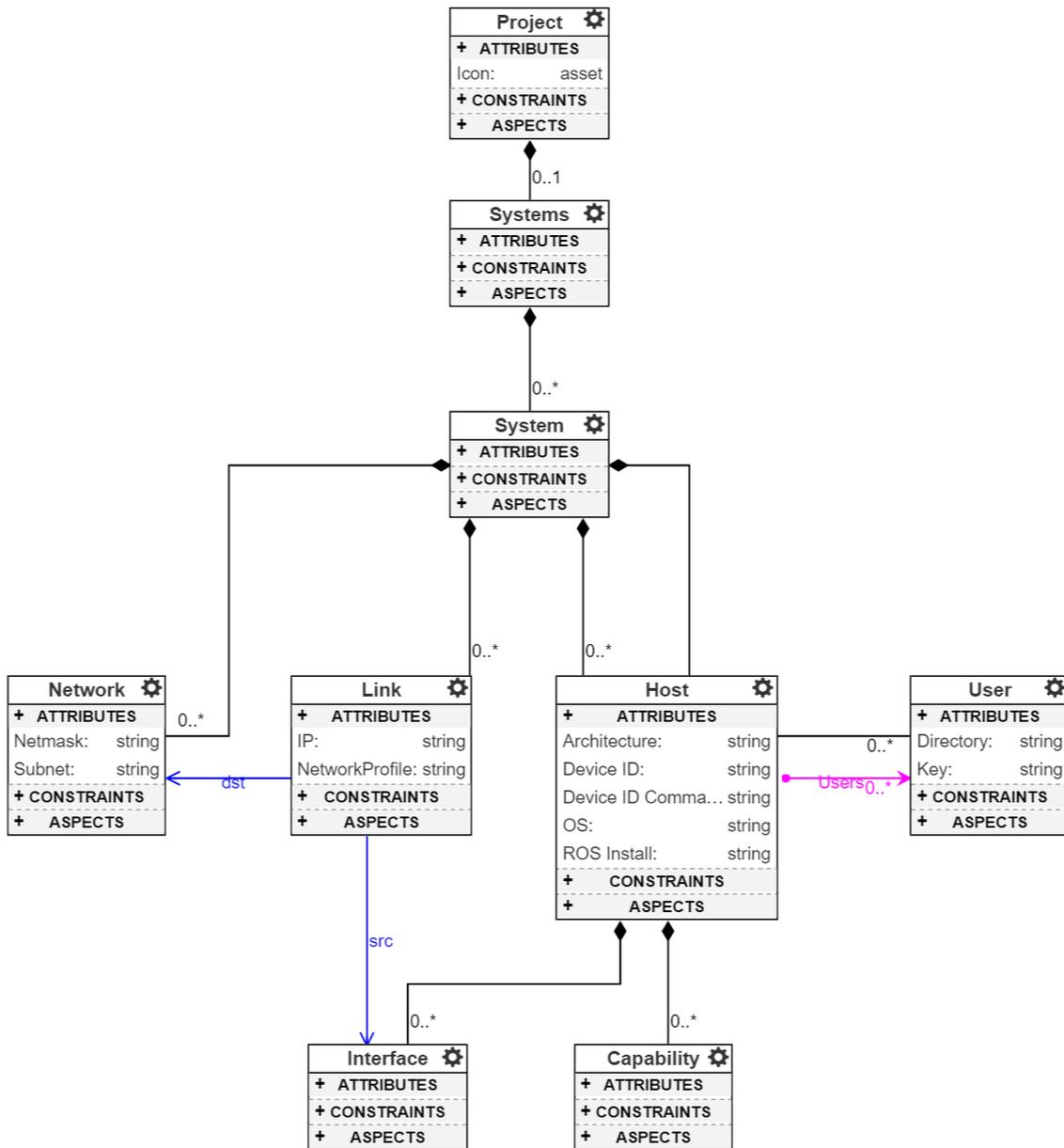
**Figure 5.** ROSMOD system hardware meta-model. System models define the hardware architectures, user roles, and networks for a (possibly distributed) CPS. A system is composed of a collection of hosts, each of which may have a different processor architecture, and each of which may have a collection of user accounts. Hosts may be connected to one or more communications networks.
