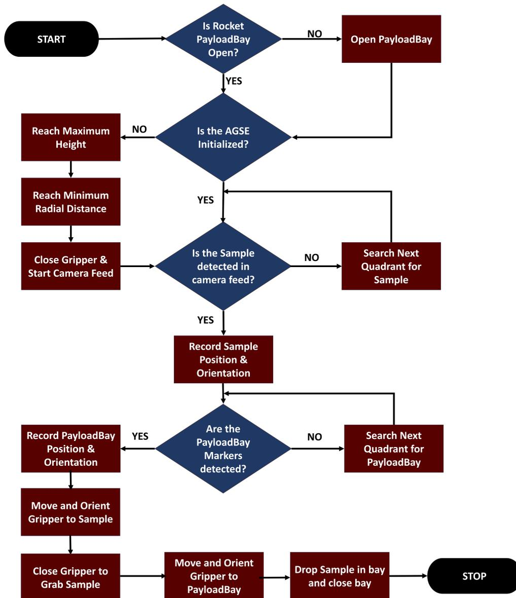
**Figure 15.** AGSE Control Flow Chart. This control flow is implemented as a state machine in the High-level control component, which uses messages and services to communicate goals and current state to the other lower-level control components.
