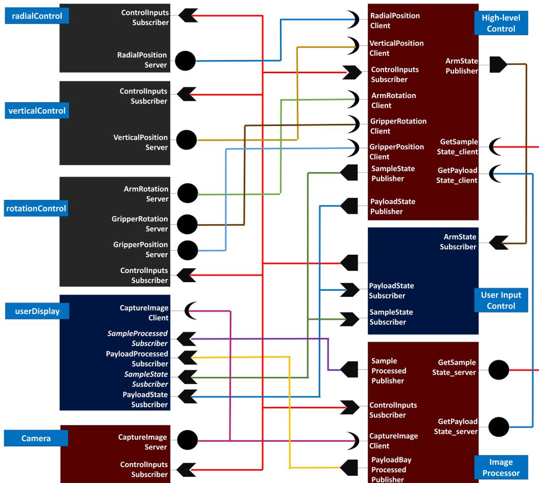
Figure 17. AGSE Component Assembly.
