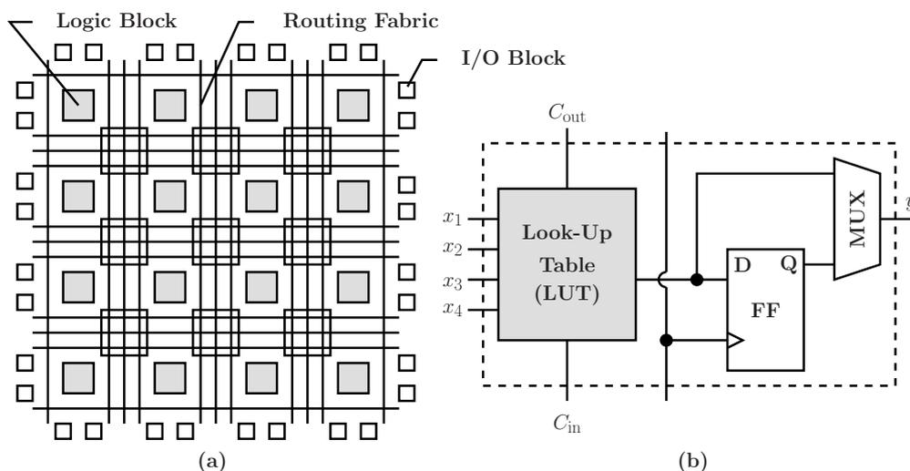
In FPGAs, LUTs are considered the basic blocks for mapping Boolean functions. Modern FPGAs allow modifications to the mapped function of LUTs through reconfiguration, partial or full, online
