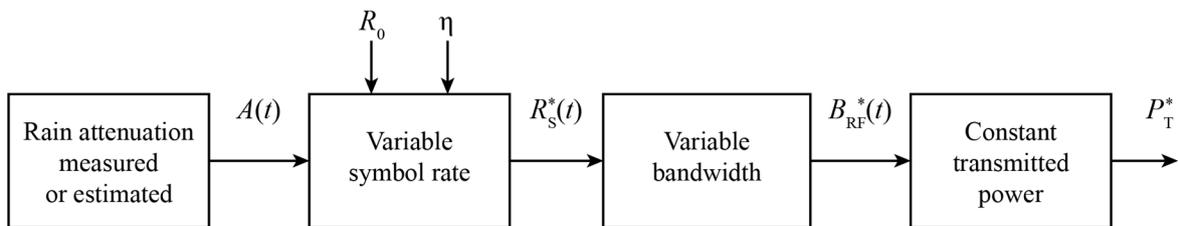
**Figure 1.** Flow-chart of the theoretical signal processing necessary for applying the method. The mathematical expressions of the symbols are given in Equations (8) and (9). The actual implementation of the processing depends on the technology of the time.
