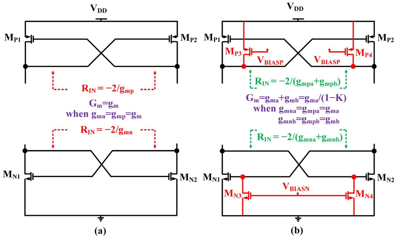
Figure 4. Approximation of the negative resistance and the condition of oscillation for (a) CVCO and (b) gm-enhanced VCO.
