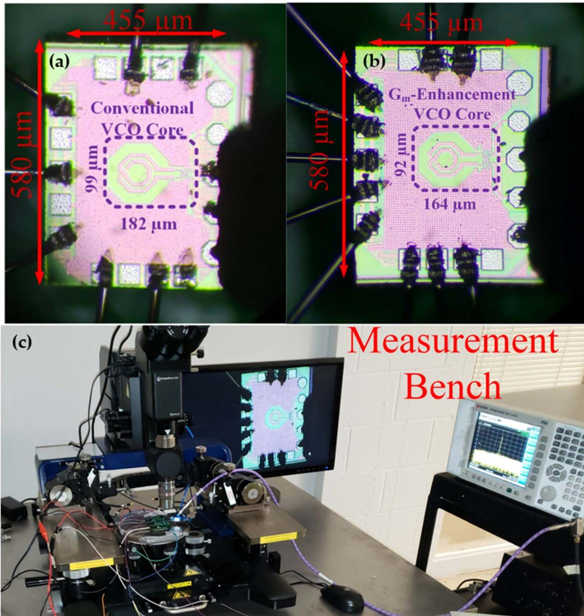
**Figure 6.** Chip micrograph of CVCO (a) and  $G_m$ -enhanced VCO (b), along with the measurement setup (c).
