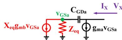
Figure 3. Negative impedance model for the proposed design.
