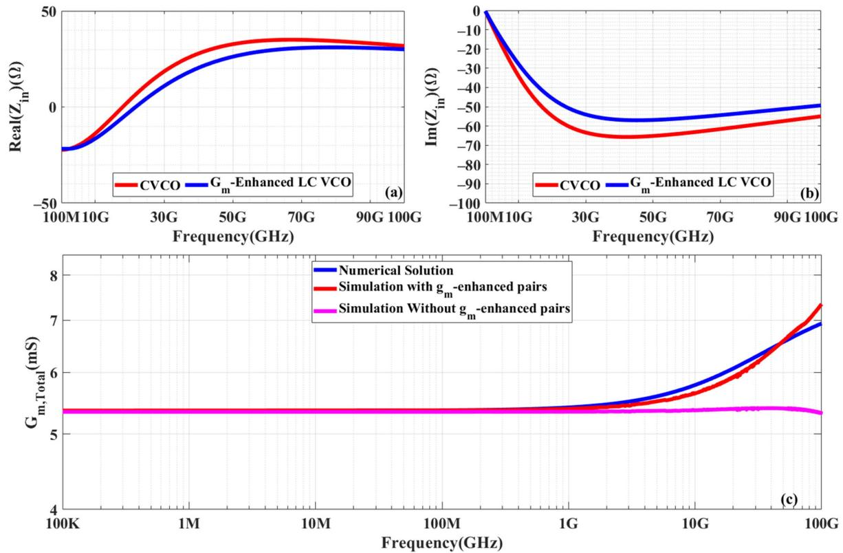
**Figure 5.** Comparison of the (a) real and (b) imaginary parts of the input impedance along with (c) the effective  $G_m$  ( $G_{m,Total}$ ) for the proposed cross-coupled pair with those of the standard cross-coupled pair across the frequency.
