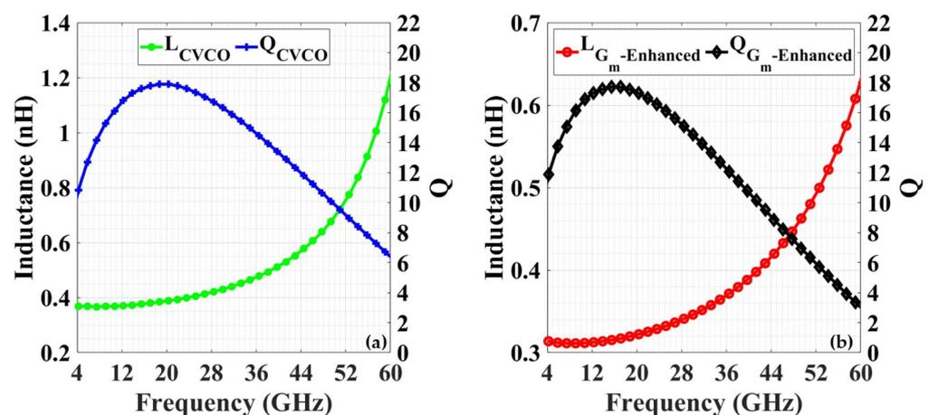
Figure 2. Q and L of inductors used in (a) CVCO and (b)  $G_m$ -enhanced VCO.
