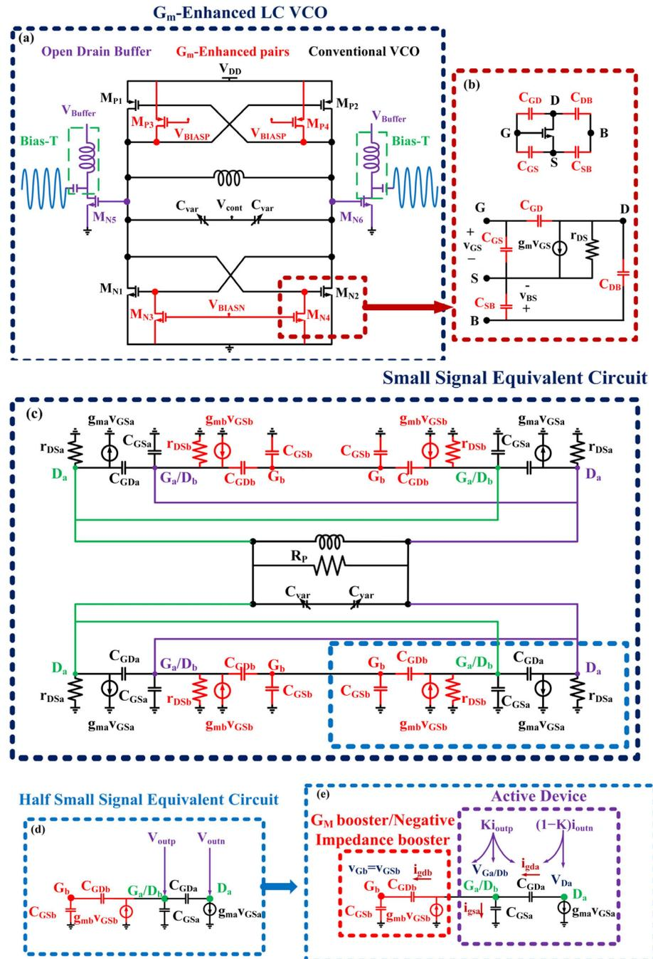
**Figure 1.** Schematic diagram of (a) the proposed  $G_m$ -enhanced CMOS LC VCO, along with the small-signal equivalent circuit (SSEC) models of the (b) MOSFET [7,17] and (c) proposed VCO. The simplified half-circuit models used for (d) the effective  $G_m$  and (e) negative impedance calculation are also shown.
