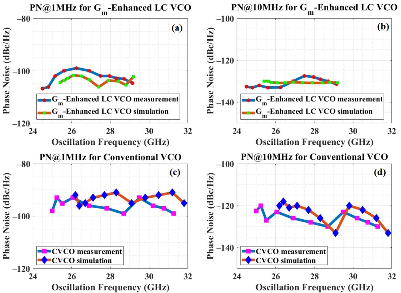
Figure 9. Measured and simulated PN of the Gm-enhanced LC VCO across the TR at (a) 1 MHz and (b) 10 MHz offset, along with the PN of the CVCO at (c) 1 MHz and (d) 10 MHz offset frequencies.
