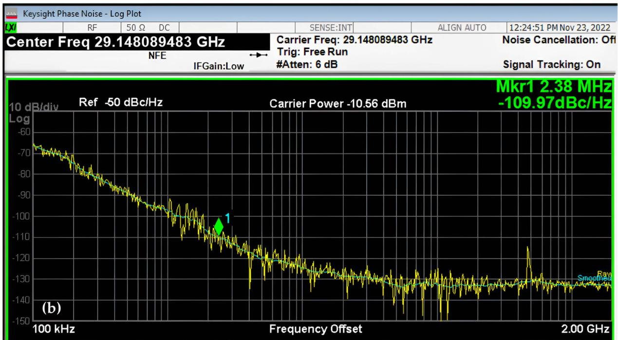
**Figure 7.** (a) The measured PN at the lower end of the tuning range for the  $G_m$ -enhanced VCO and CVCO after de-embedding, and the frequency spectrum of the  $G_m$ -enhanced VCO, along with (b) the measured PN performance of the  $G_m$ -enhanced VCO at the upper end of the tuning range before de-embedding.
