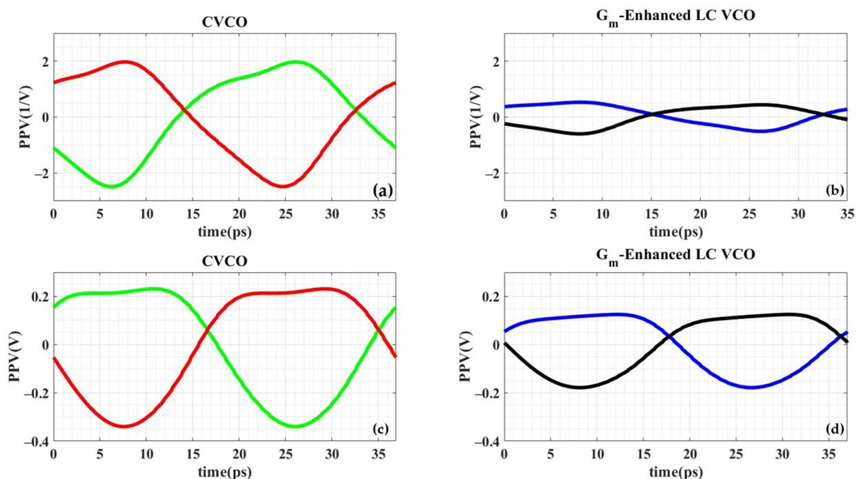
**Figure 10.** PPV results for differential outputs (green and red for CVCO, blue and black for  $G_m$ -enhanced LC VCO): HBnoise results for (a) CVCO and (b)  $G_m$ -enhanced LC VCO; HB results for (c) CVCO and (d)  $G_m$ -enhanced LC VCO.
