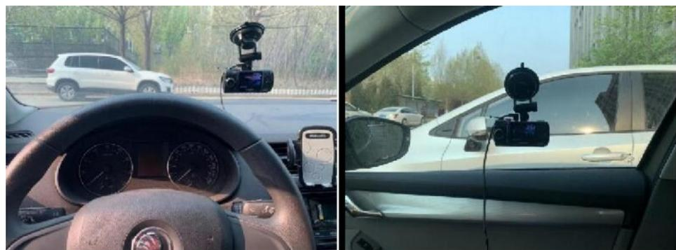
**Figure 3.** Dash camera placement. Dash cameras were placed in two locations to collect data from the front and from the side.
