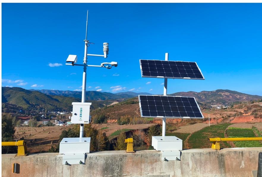
**Figure 2.** Self-developed traffic meteorological data collection equipment.
