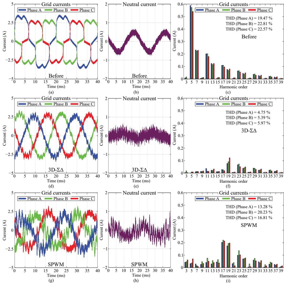
**Figure 10.** Experimental results. (a–c) Before filtering and balancing. (d–f) After filtering and balancing using 3D-ΣΔ. (d–f) After filtering and balancing using SPWM. (a,d,g) Grid current waveforms. (b,e,h) Neutral current waveforms. (c,f,i) Grid currents in frequency domain.
