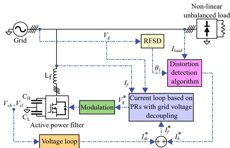
**Figure 5.** Overall block diagram control of the active power filter.
