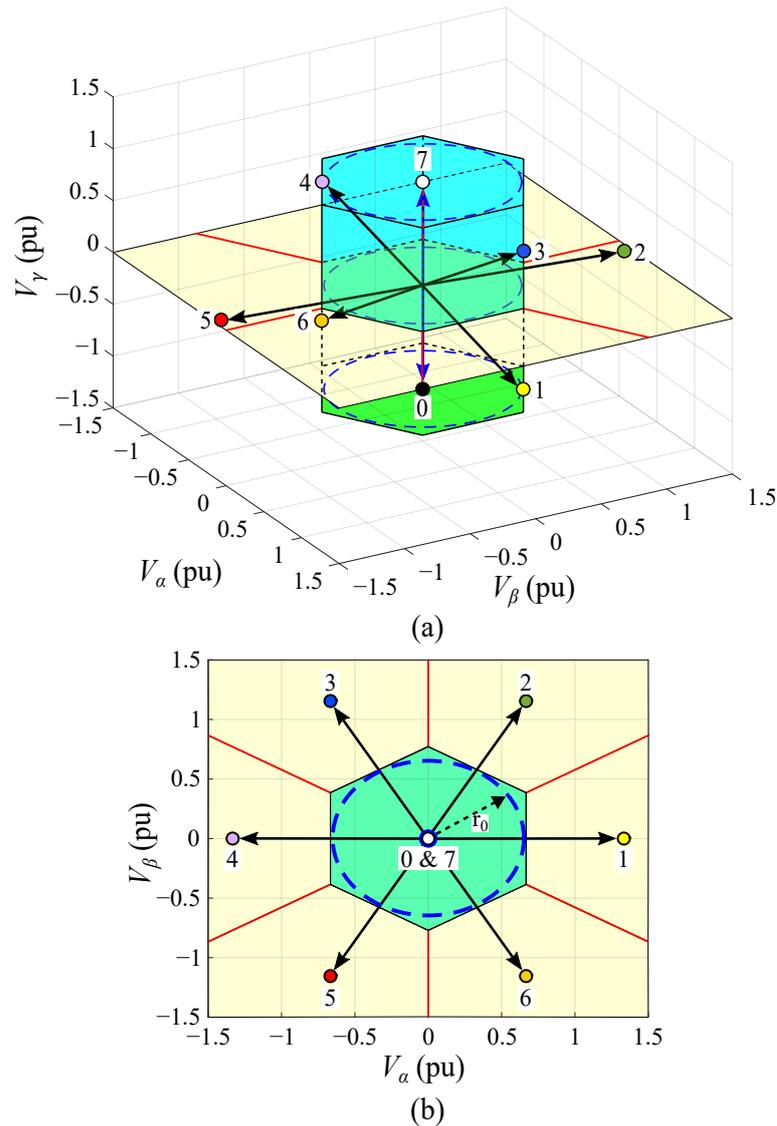
**Figure 3.** Two-level, three-phase converter switching states: (a) isometric view and (b) view from the zero-sequence axis.
