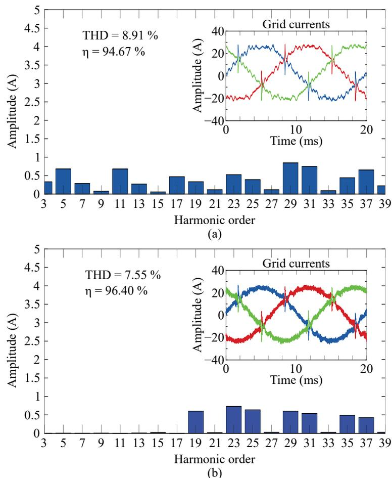
**Figure 7.** Simulated grid currents when the active power filter is compensating for harmonics and balancing the grid using different modulation strategies: (a) SPWM and (b) 3D- $\Sigma\Delta$ .
