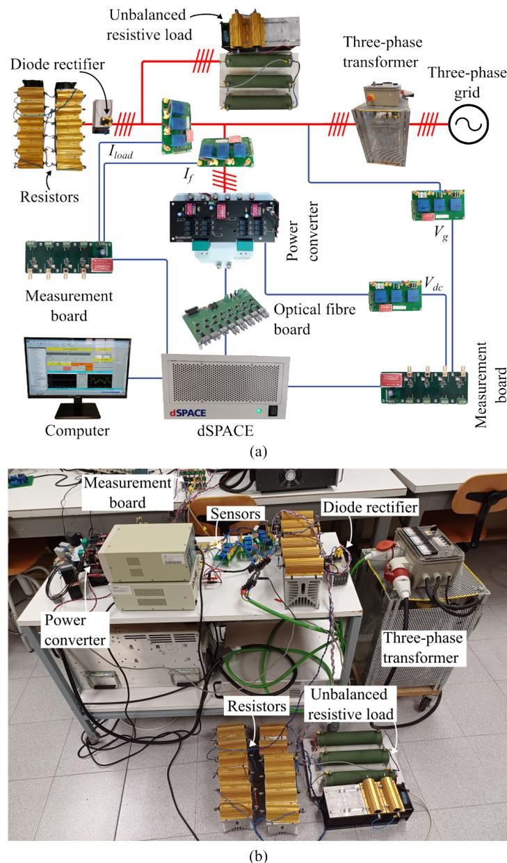
Figure 9. View of the experimental setup: (a) schematic; (b) photographic depiction.
