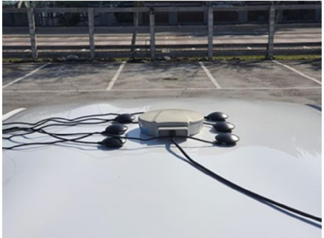
Figure 2. All GPS receivers are mounted on the vehicle.
