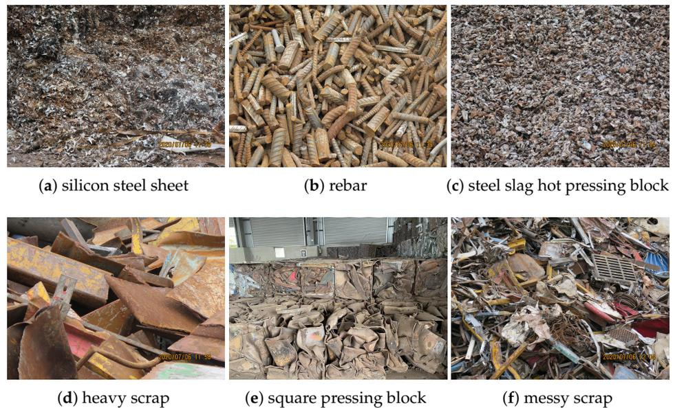
**Figure 2.** Examples of different scrap types in self-built datasets.
