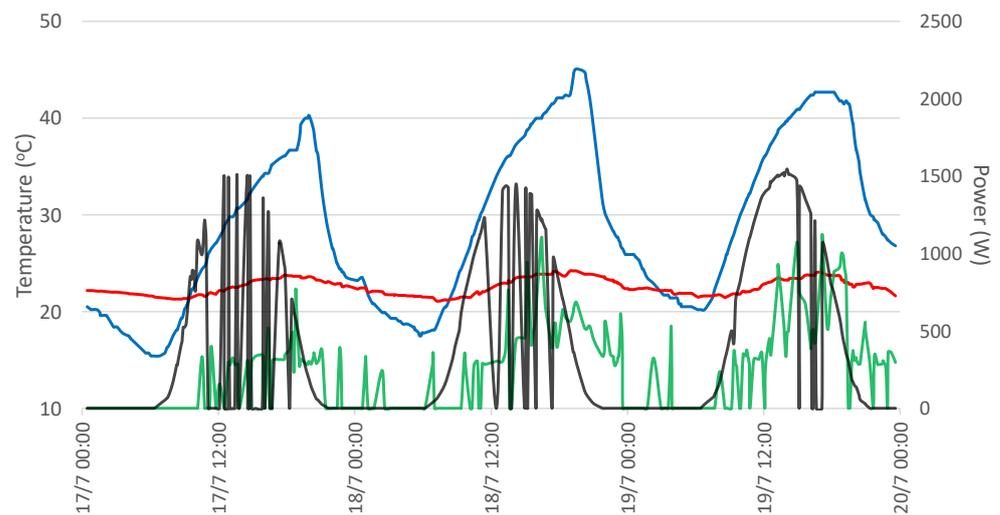
**Figure 7.** Sample data recorded with external temperature (blue) and temperature inside the model house (red), photovoltaic power (black), and heat pump electrical power consumption (green) for 17 to 19 July.
