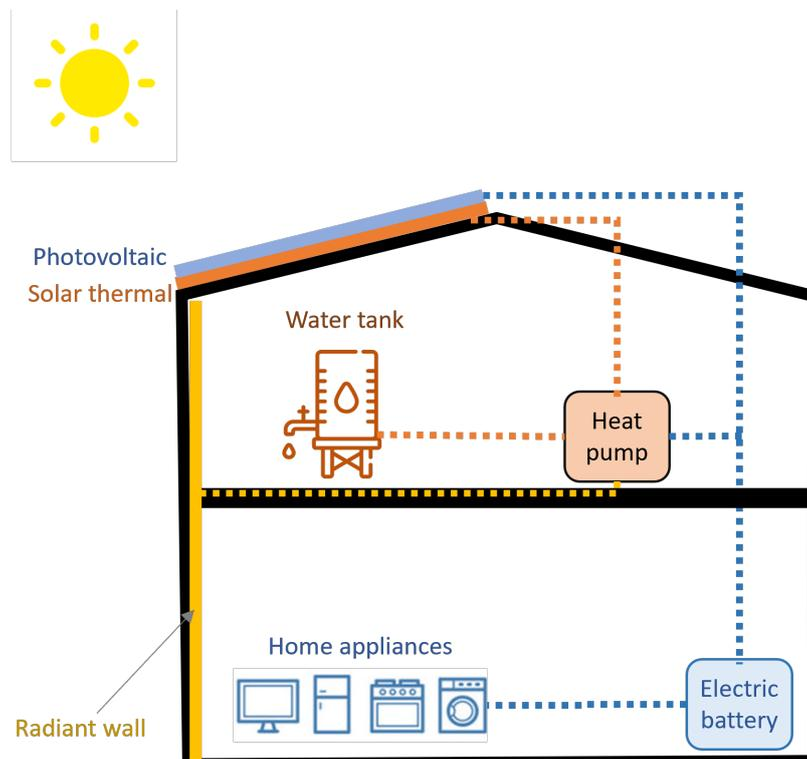
**Figure 1.** Self-sufficient energy system.
