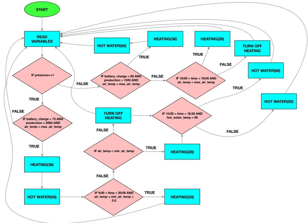
Figure 3. Example of an automatic control algorithm for efficient winter heating management.
