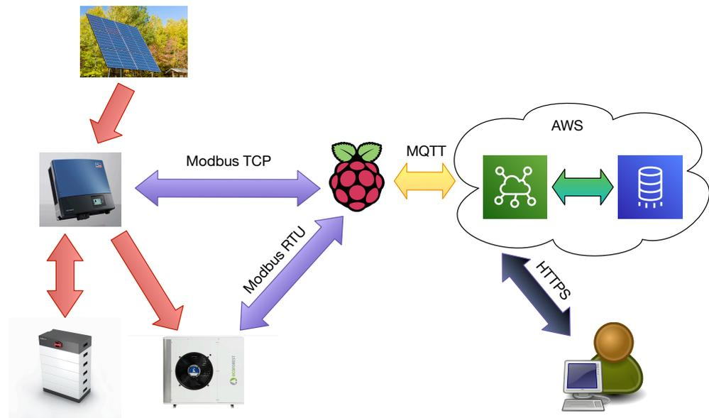
**Figure 2.** System diagram.
