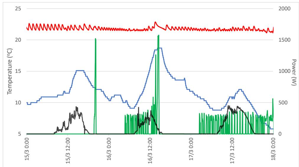
**Figure 6.** Sample data recorded with external temperature (blue) and temperature inside the model house (red), photovoltaic power (black), and heat pump electrical power consumption (green) for 15 to 17 March.
