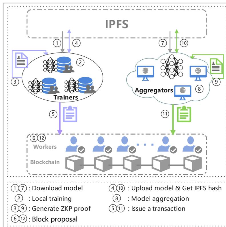
Figure 3. The roles and components of the ZKP-based TrustDFL framework assisted by blockchain.
