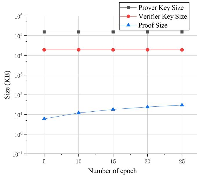
Figure 6. Storage overhead of ZKP for local training with different epoch numbers.
