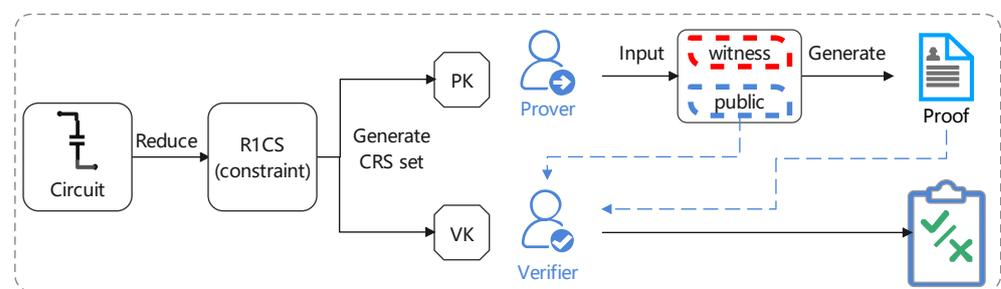
**Figure 2.** The construction process of the zk-SNARK.
