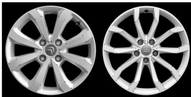
Figure 3. Labeled samples. All samples were labelled using LabelMe to extract feature points on either side of each spoke. In the central area, the position where the trend of the spokes changes was used as the endpoint.
