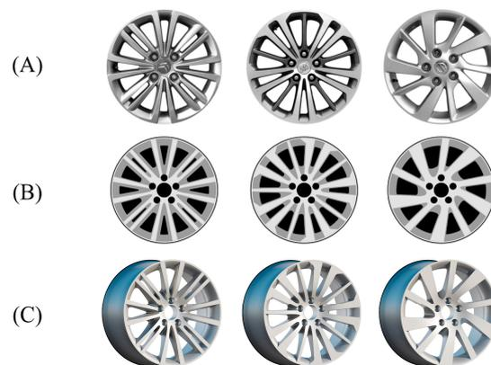
**Figure 14.** Results of the reconstruction of wheel hub shape. (A) Original sample. (B) Generated 2D shapes. (C) Constructed 3D models.
