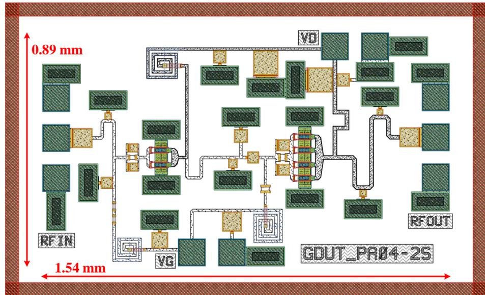
Figure 16. Complete layout of the 24–30 GHz GaN MMIC PA, chip size (including dicing streets):  $1.8 \times 1.1 \text{ mm}^2$ .
