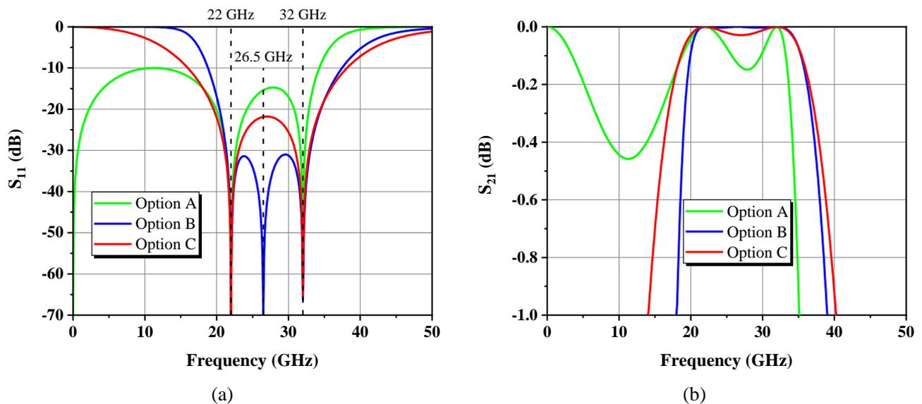
**Figure 7.** Ideal frequency responses of compensators: (a)  $S_{11}$ ; (b)  $S_{21}$ .
