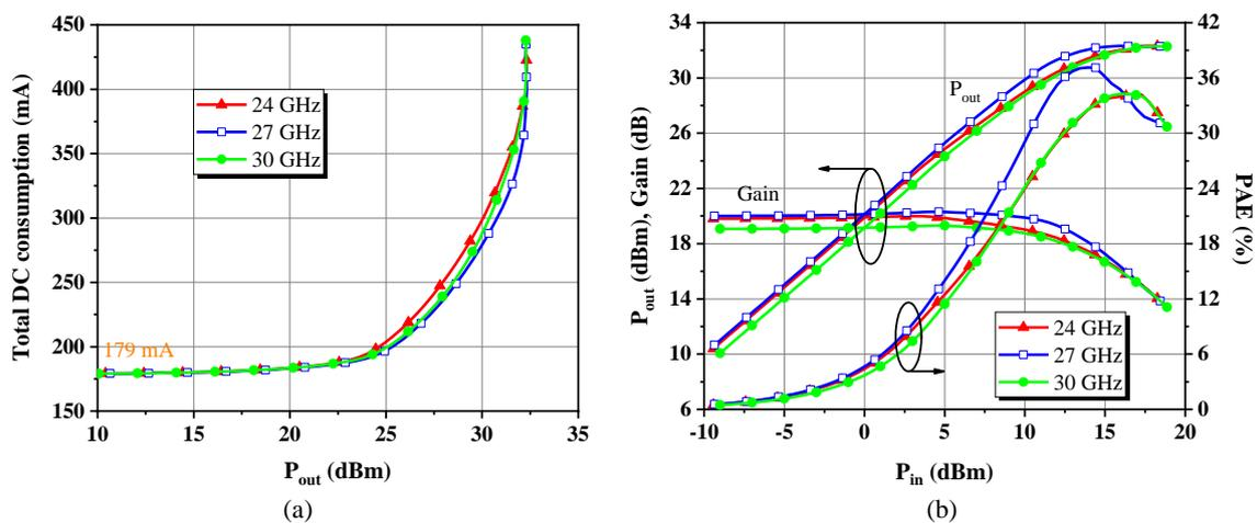
Figure 18. Simulated (a) total DC consumption versus  $P_{out}$ , (b)  $P_{out}$ , PAE, and gain behaviors with respect to  $P_{in}$  at three discrete frequencies.
