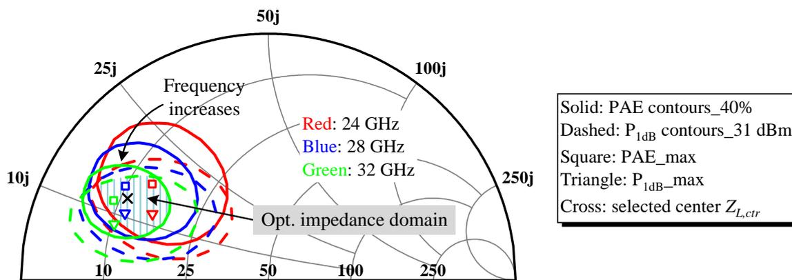
Figure 2. Simulated load-pull contours at  $P_{1dB}$  for the output stage cell.
