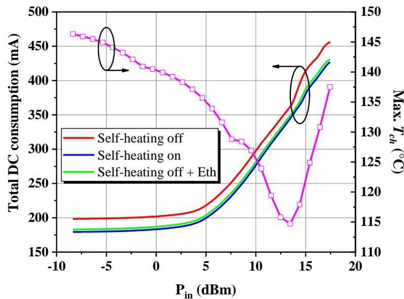
Figure 20. Total DC consumption and steady-state maximum channel temperature within the chip evaluated for different  $P_{in}$  at  $f_0$ .
