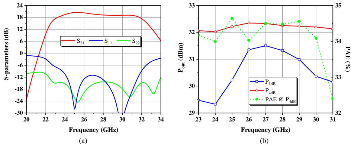
Figure 17. Simulated (a) S-parameters, (b)  $P_{out}$ , and PAE at 4 dB gain compression.
