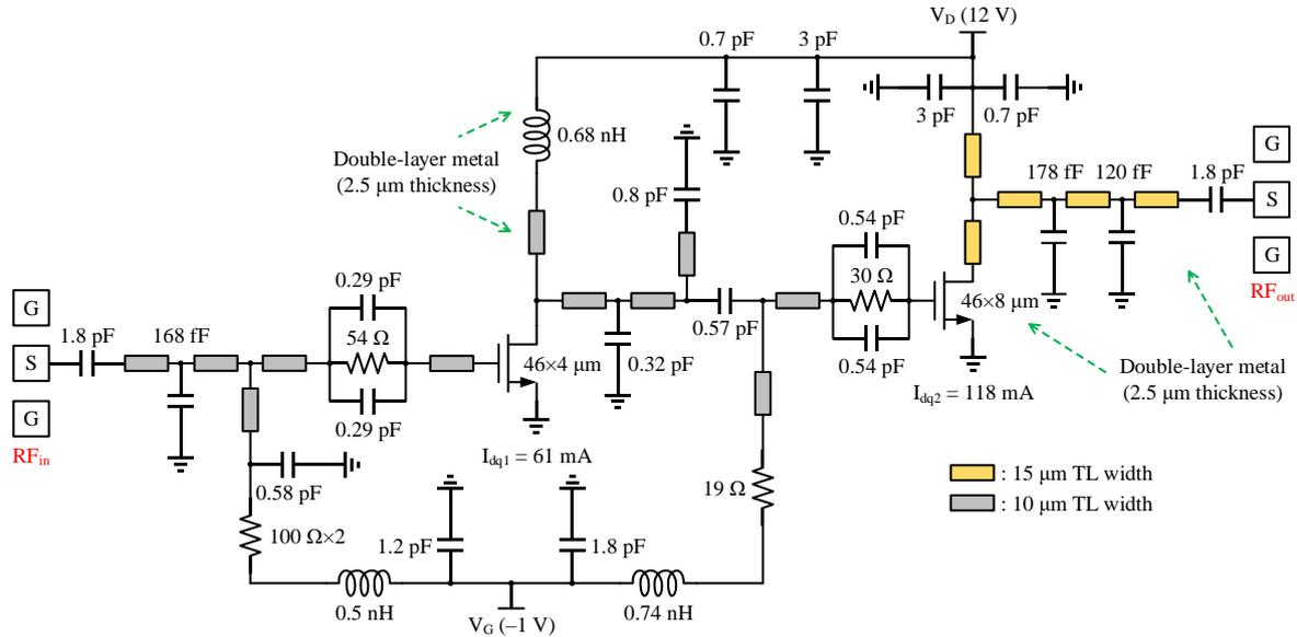
Figure 15. Schematic diagram of the two-stage PA.
