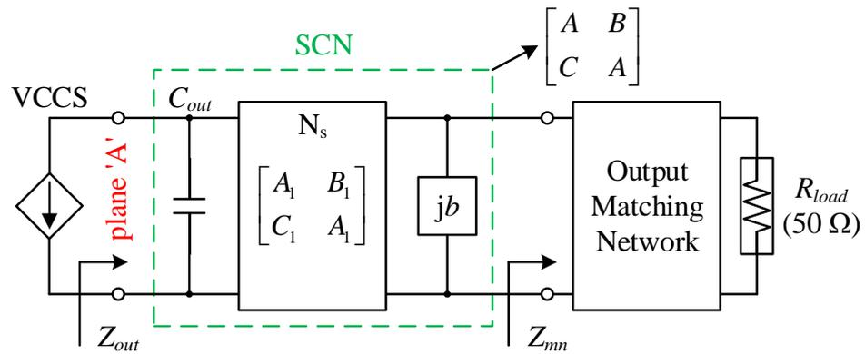
Figure 4. Output circuit composed of SCN and OMN.
