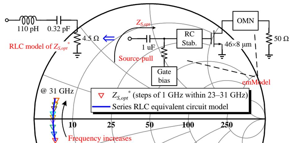
Figure 10. Impedance distribution of  $Z_{S,opt}^*$  and its series RLC equivalent circuit.
