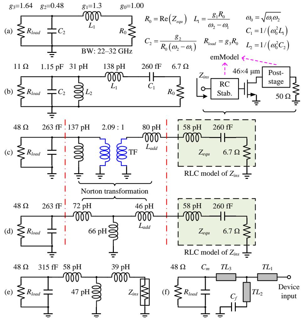
**Figure 14.** IMN design flow: (a) LP prototype after impedance and frequency scaling; (b) converted BP version; (c) upward IT of  $R_{load}$  to  $48 \Omega$ ; (d) Norton transformation to remove the ideal transformer; (e) network optimization for realistic  $Z_{ins}$ ; (f) corresponding ultimate IMN in mixed-element form.
