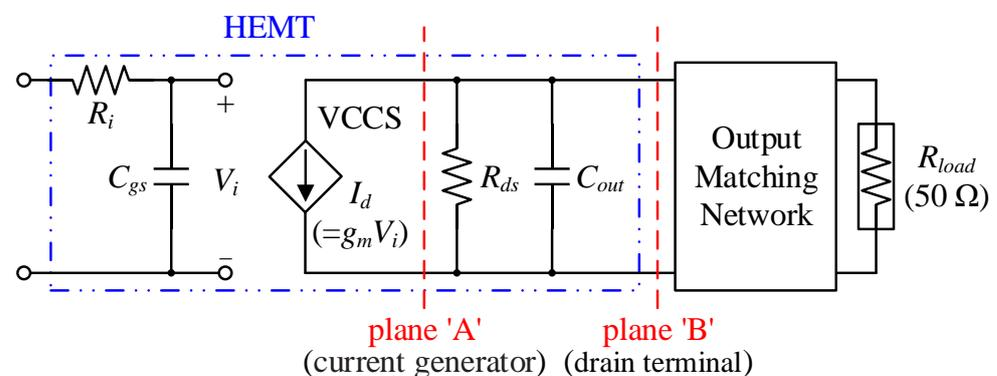
Figure 1. Simplified equivalent circuit model of an HEMT.
