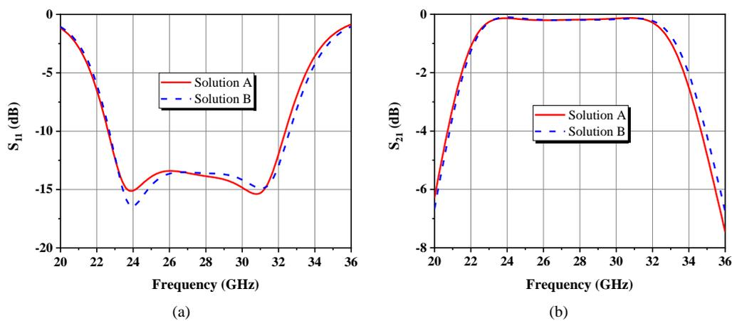
Figure 13. Ideal frequency response of ISMN in solution A and B cases: (a)  $S_{11}$ ; (b)  $S_{21}$ .
