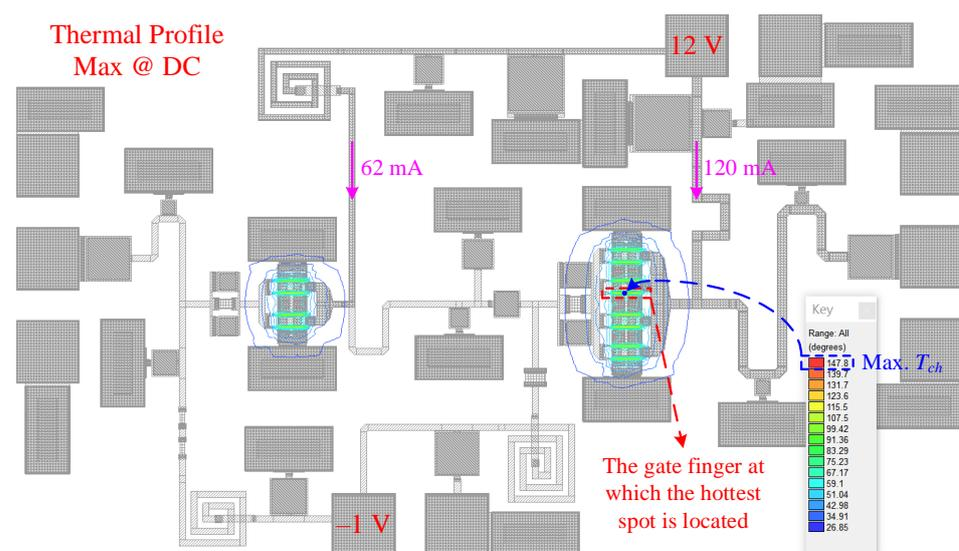
**Figure 19.** Two-dimensional (2D) thermal map of the designed MMIC at a backside temperature of 26.85 °C obtained from ADS HeatWave.
