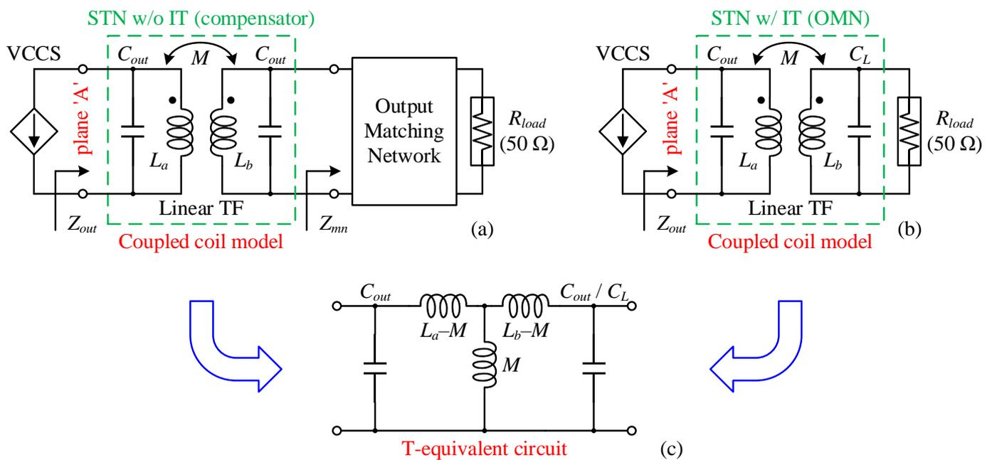
Figure 5. STNs (a) without and (b) with IT function and (c) their AC-equivalent circuits.
