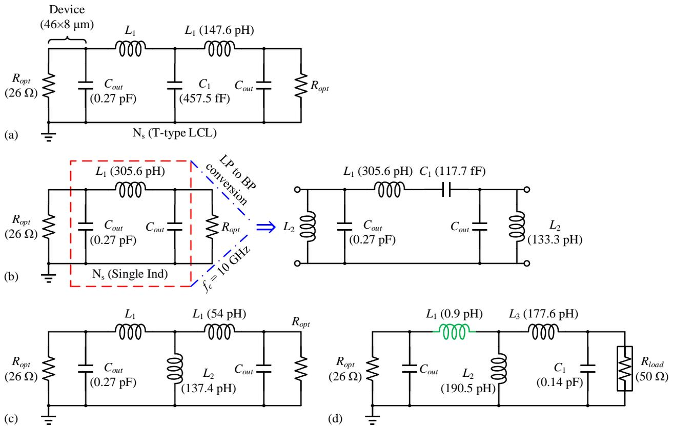
**Figure 6.** (a) LP compensator with  $N_s$  of T-type LCL topology. (b) BP compensator converted from an LP SCN with three lumped elements. (c) STN as a compensator only. (d) STN capable of realizing the transformation from  $R_{load}$  to  $R_{opt}$ .
