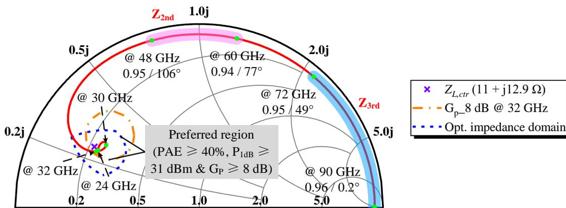
Figure 9. EM-simulated transformation feature ( $S_{11}$ ) of OMN from 22 to 90 GHz.
