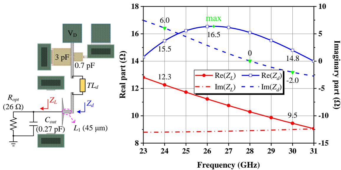
**Figure 8.** Illustration and results of reactance compensation for the output impedance of a  $46 \times 8 \mu\text{m}$  power cell using a shorted stub.
