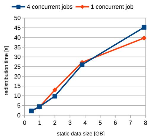
**Figure 8.** Redistribution time against static data size for the sPS pipeline.
