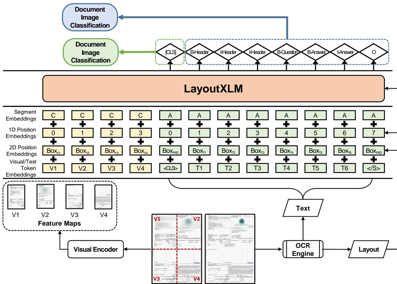
Figure 4. Structure of the unstructured document image understanding model (LayoutXML).
