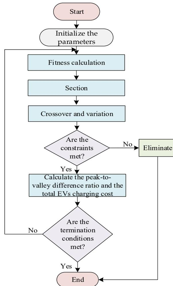
**Figure 2.** Flow chart of elite genetic algorithm (EGA).
