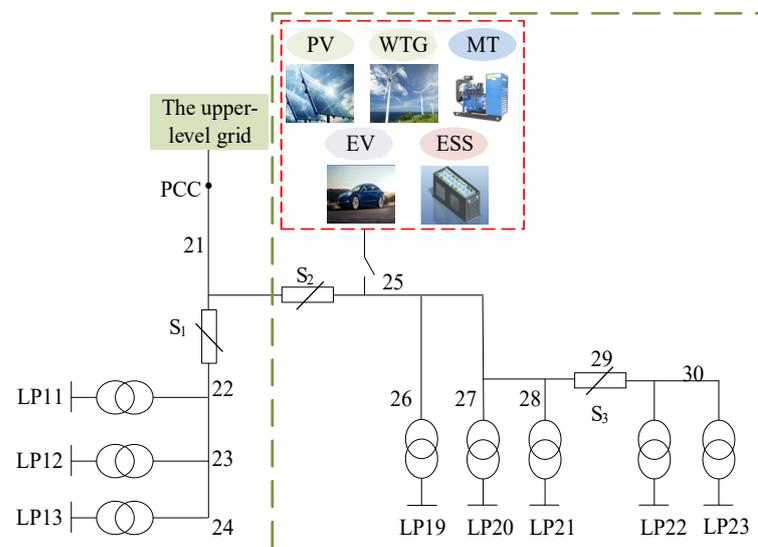
**Figure 3.** The microgrid system with a microturbine (MT), wind turbine generator (WTG), photovoltaics (PVs), electric vehicles (EVs), an energy storage system (ESS), and loads.
