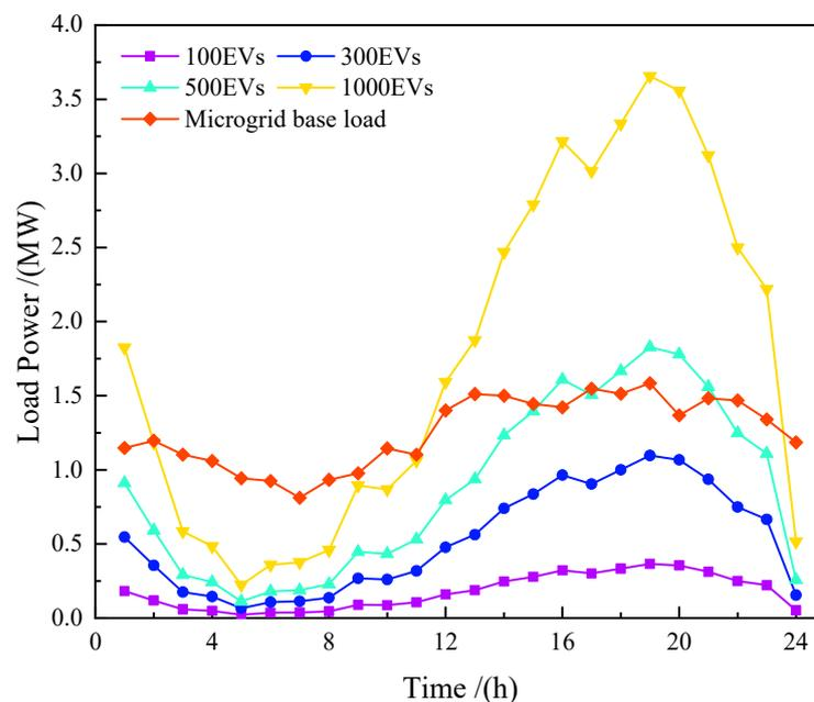
**Figure 4.** Microgrid base load curve and load curve of different numbers of EVs in one day.
