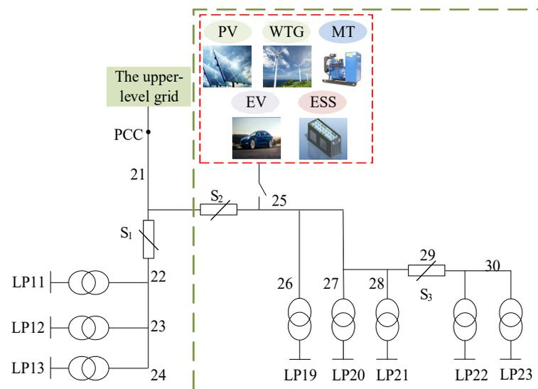
**Figure 3.** The microgrid system with a microturbine (MT), wind turbine generator (WTG), photovoltaics (PVs), electric vehicles (EVs), an energy storage system (ESS), and loads.
