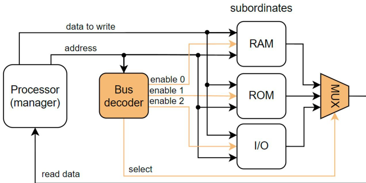
Figure 3. Simplified block diagram of a system with AMBA AHB bus.
