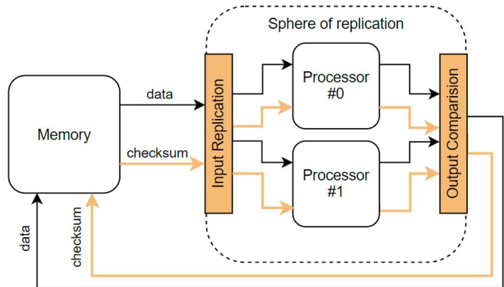
Figure 1. Sphere of replication and protected memory.
