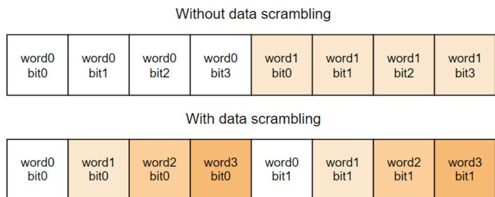
**Figure 2.** Example of data in memory with and without data scrambling.
