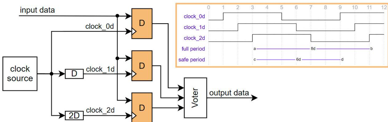
**Figure 4.** Temporal redundancy with delay (D) in the replicated clock signals.
