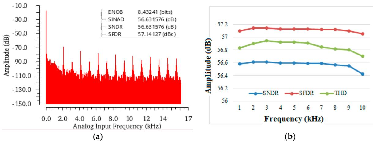
Figure 10. (a) Simulated dynamic performance FFT spectrum. (b) Dynamic performance vs. input frequency.
