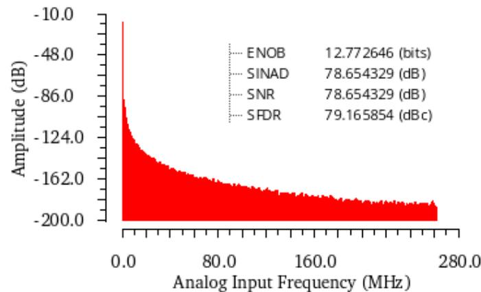
Figure 4. FFT spectrum plot of novel bootstrap switch.
