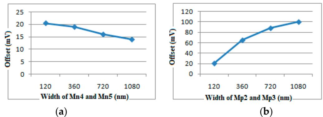
Figure 6. Simulation of offset rendered by each transistor.
