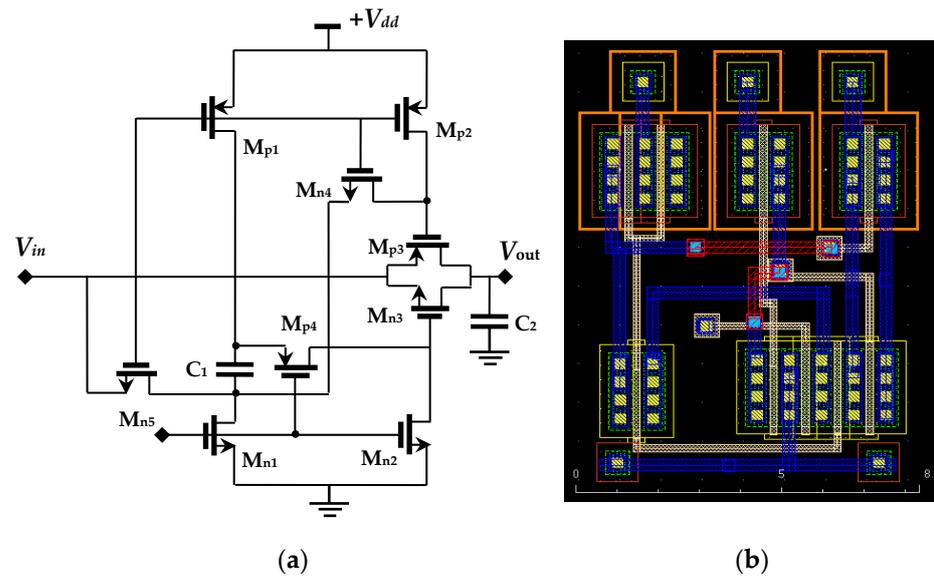
Figure 2. (a) Proposed bootstrap switch and (b) its layout.
