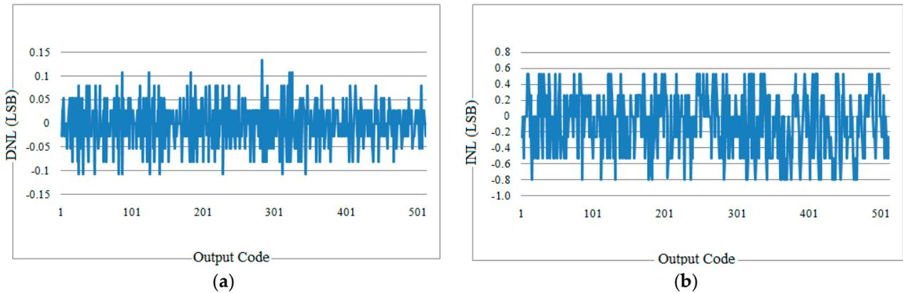
Figure 9. Linearity error of (a) DNL and (b) INL.
