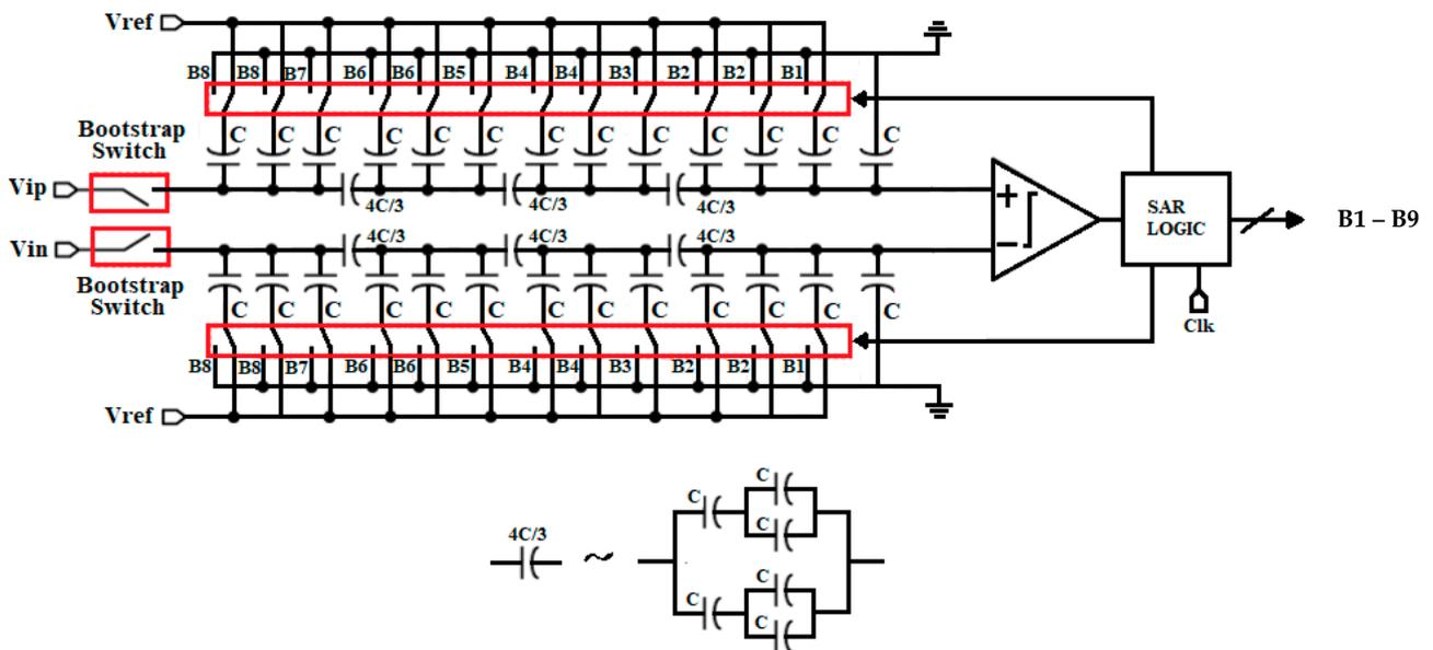
Figure 1. Proposed fully differential SAR ADC.
