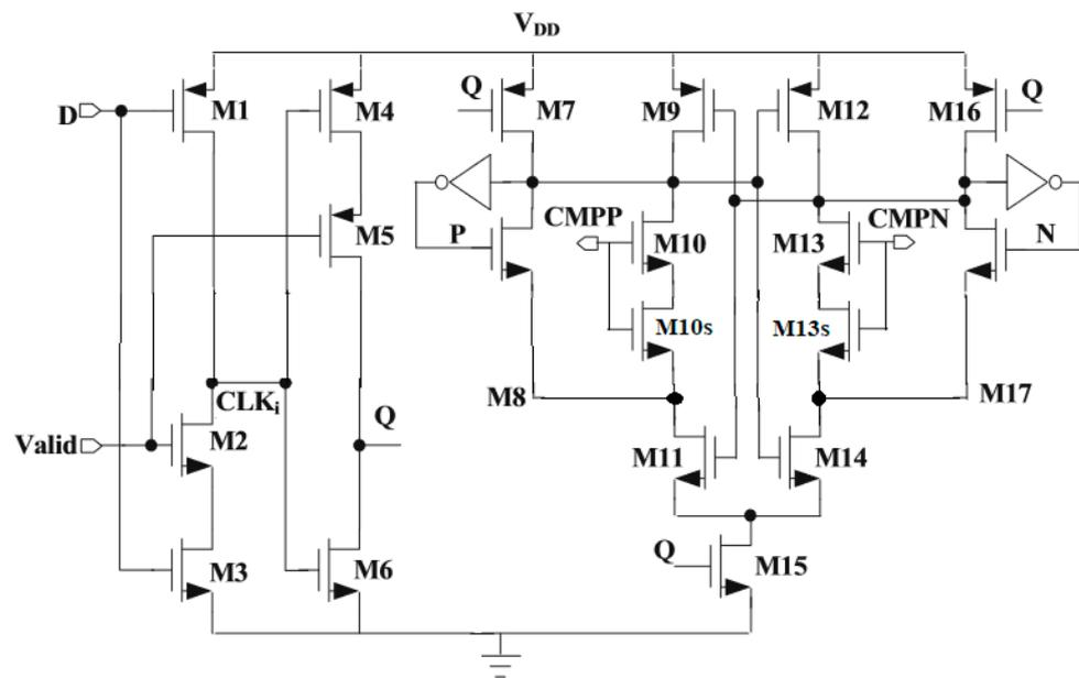
Figure 8. Modified SAR control logic.
