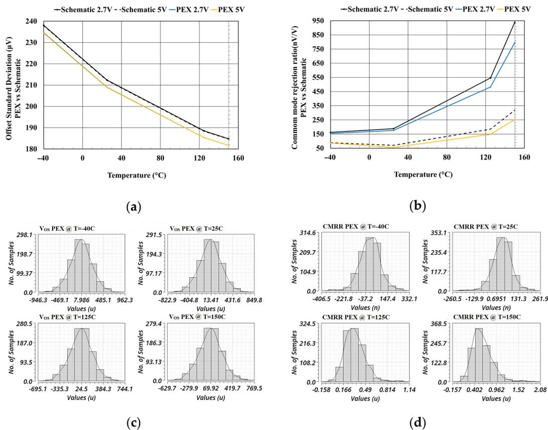
**Figure 17.** Parasitic extraction simulation results. (a) Offset standard deviation comparison; (b) common-mode rejection ratio standard deviation comparison; (c)  $V_{OS}$  histograms at different temperatures,  $V_{DD} = 5$  V; (d) CMRR histograms at different temperatures,  $V_{DD} = 5$  V.
