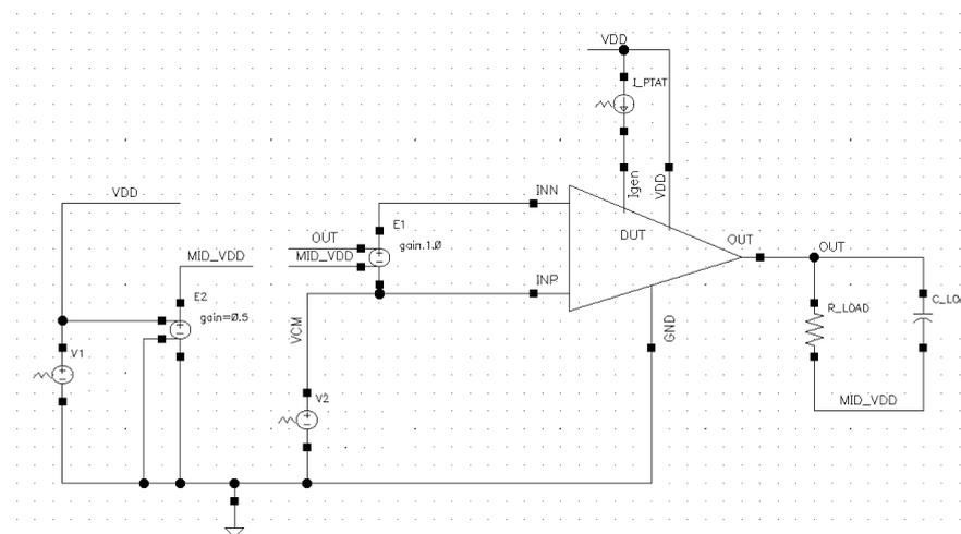
**Figure 6.** DC parameter evaluation testbench.
