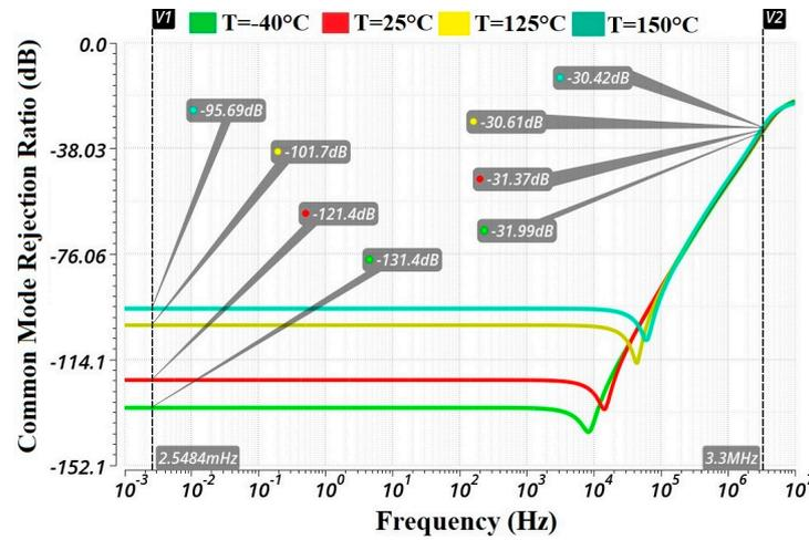
Figure 21. CMRR frequency response at different temperatures.
