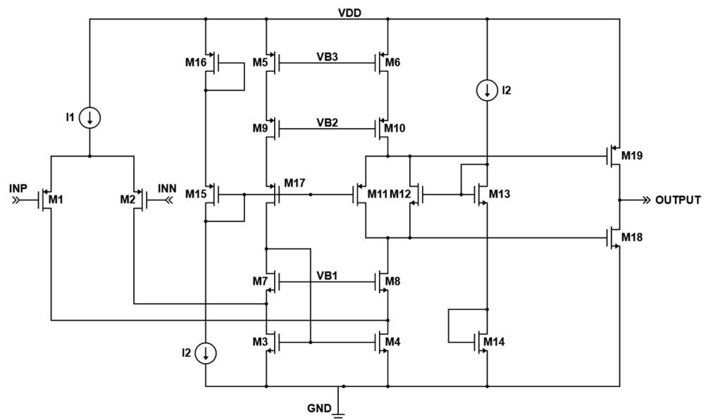
Figure 2. Two stage op-amp with folded cascode.
