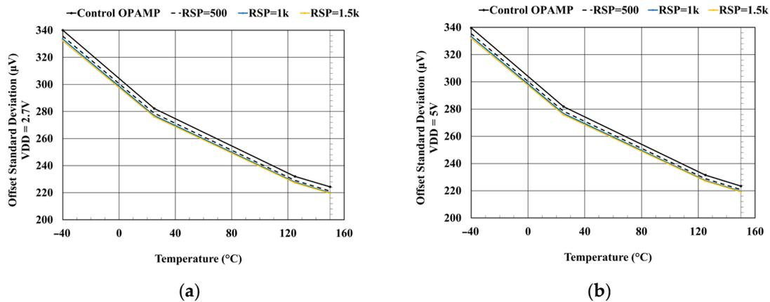
**Figure 7.** Offset voltage standard deviation distribution versus temperature, with  $RS3 = RS4 = RSP$  (considered a parameter) and  $RS1 = RS2 = RSN = 0 \Omega$ . (a)  $VDD = 2.7 V$ ; (b)  $VDD = 5 V$ .
