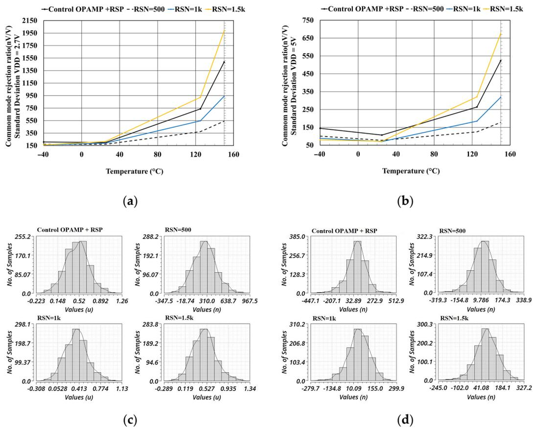
**Figure 12.** Common-mode rejection ratio deviation distribution versus temperature, with  $R_{S3} = R_{S4} = R_{SP} = 1 \text{ k}\Omega$  and  $R_{S1} = R_{S2} = R_{SN}$  (considered a parameter). (a)  $V_{DD} = 2.7 \text{ V}$ ; (b)  $V_{DD} = 5 \text{ V}$ ; (c) Monte Carlo histograms,  $T = 27 \text{ }^\circ\text{C}$ — $V_{DD} = 2.7 \text{ V}$ ; (d) Monte Carlo histograms,  $T = 27 \text{ }^\circ\text{C}$ — $V_{DD} = 5 \text{ V}$ .
