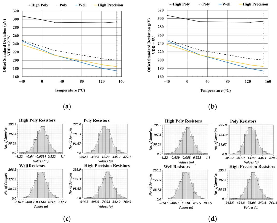
**Figure 15.** Offset voltage standard deviation distribution versus temperature with different resistor types implemented. (a) VDD = 2.7 V; (b) VDD = 5 V; (c) Monte Carlo histograms, T = 27 °C—VDD = 2.7 V; (d) Monte Carlo histograms, T = 27 °C—VDD = 5 V.
