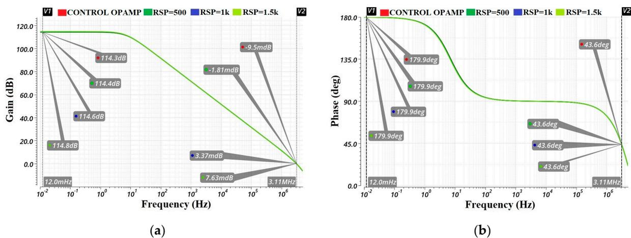
Figure 10. Bode plot waveforms for  $RS_3 = RS_4 = RSP$  (considered parameters) and  $RS_1 = RS_2 = RSN = 0 \Omega$ . (a) Gain waveforms; (b) phase waveforms.
