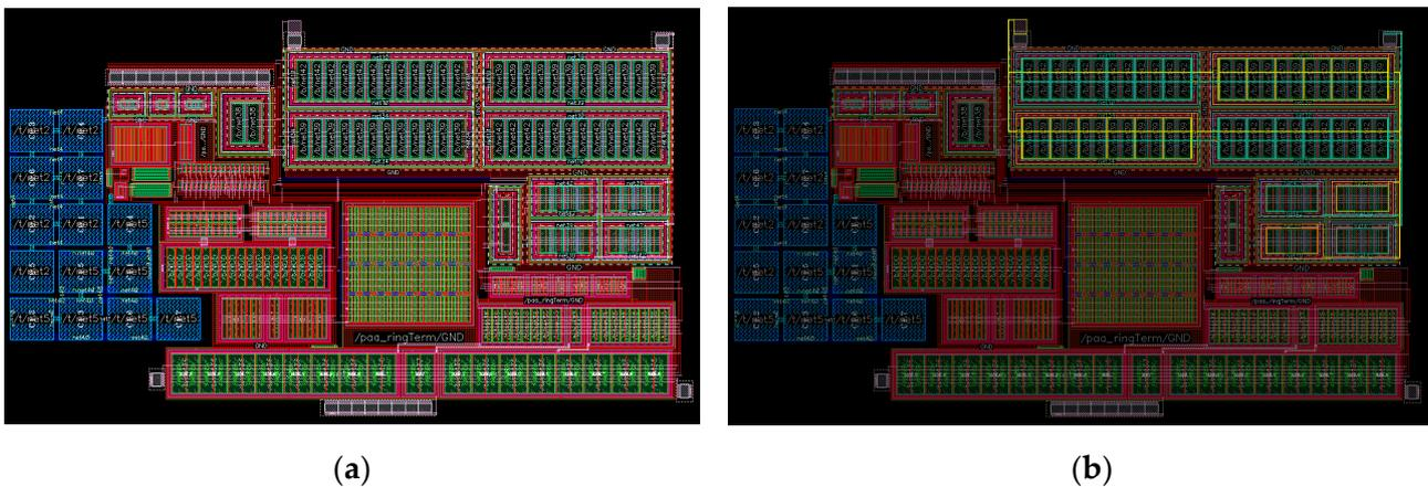
**Figure 22.** Proposed circuit layout, with  $R_{S1} = R_{S2} = 1.5 \text{ k}\Omega$ , and  $R_{S3} = R_{S4} = 1 \text{ k}\Omega$ . (a) Overview; (b) resistor wire matching for offset reduction.
