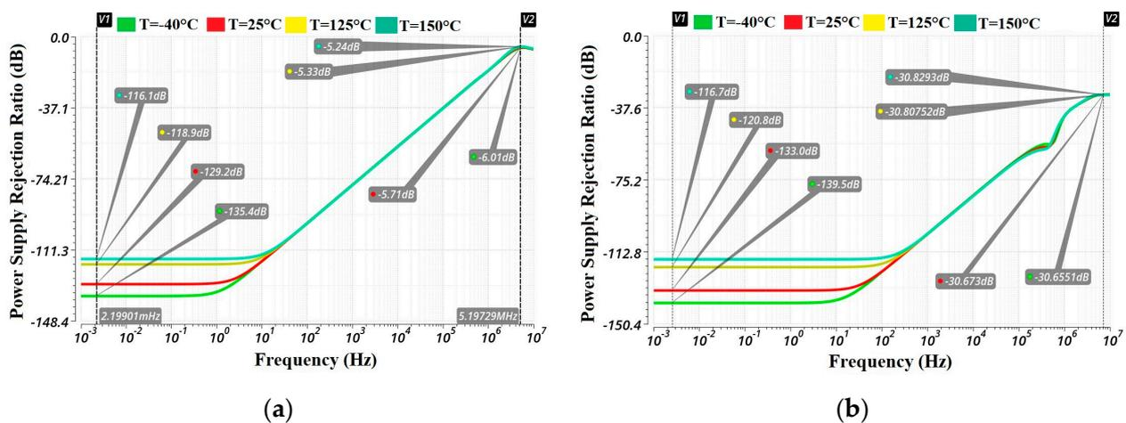
Figure 20. Frequency response at different temperatures (a)  $PSRR_+$ ; (b)  $PSRR_-$ .
