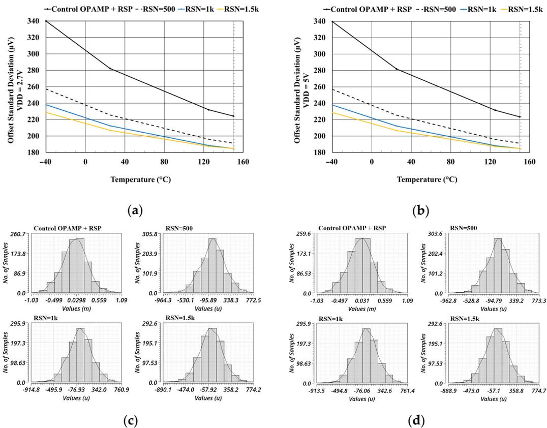
**Figure 11.** Offset standard deviation distribution versus temperature, with  $R_{S3} = R_{S4} = R_{SP} = 1\text{ k}\Omega$  and  $R_{S1} = R_{S2} = R_{SN}$  (considered a parameter). (a)  $V_{DD} = 2.7\text{ V}$ ; (b)  $V_{DD} = 5\text{ V}$ ; (c) Monte Carlo histograms,  $T = 27\text{ }^\circ\text{C}$ — $V_{DD} = 2.7\text{ V}$ ; (d) Monte Carlo histograms,  $T = 27\text{ }^\circ\text{C}$ — $V_{DD} = 5\text{ V}$ .
