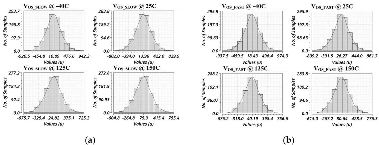
**Figure 18.** Parasitic extraction histogram results in corners for offset voltage: (a) slow; (b) fast.
