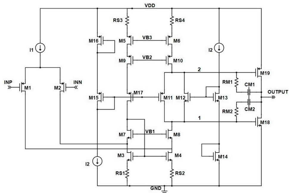
Figure 5. Proposed low-offset-voltage two-stage folded-cascode current-mirror source degeneration op-amp.
