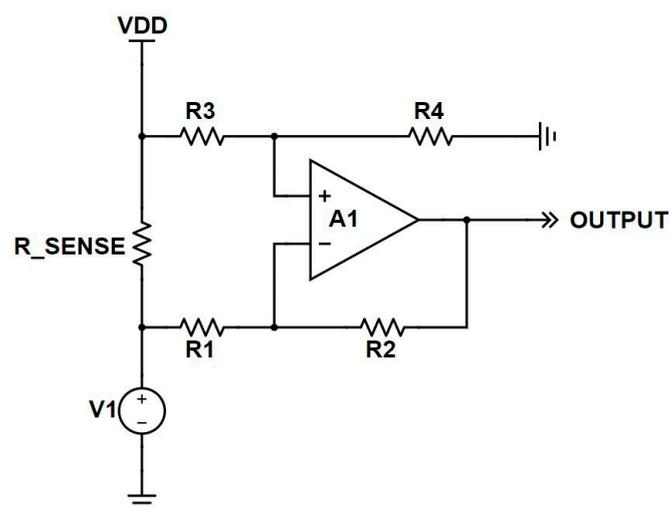
Figure 1. Unidirectional high-side current-sense-circuit schematic.
