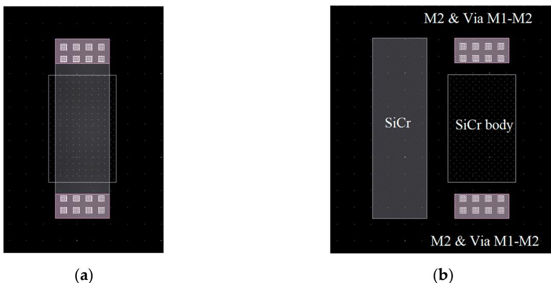
**Figure 23.** SiCr layout implementation. (a) Layout view; (b) layer masks used.
