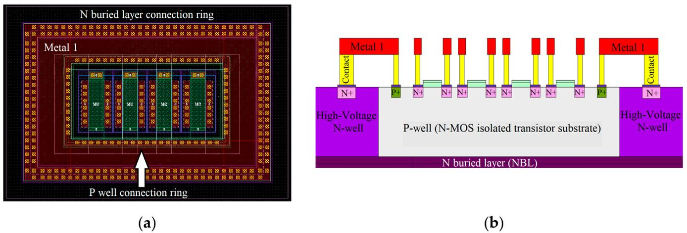
Figure 24. Isolated nMOS transistor. (a) Layout view; (b) cross-section.
