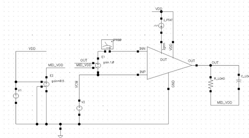
Figure 9. UGBW, phase margin and gain testbench schematic.
