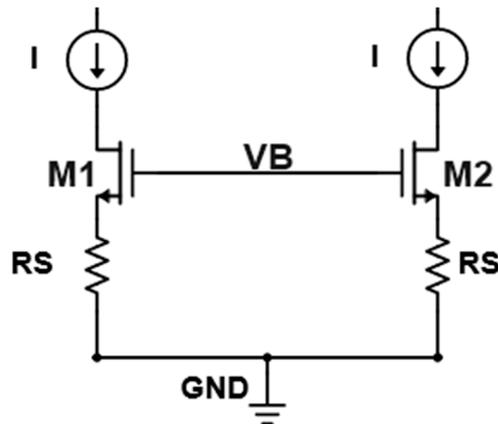
Figure 4. Current mirror with source degeneration implemented.
