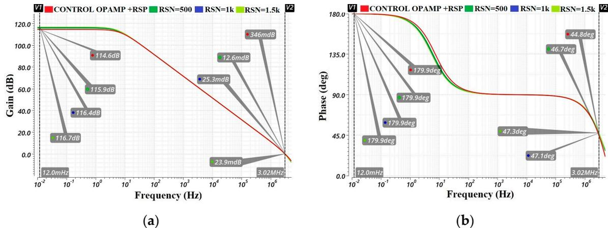
**Figure 16.** Bode plot waveforms for RS3 = RS4 = RSP = 1 kΩ and RS1 = RS2 = RSN (considered parameters). (a) Gain waveforms; (b) phase waveforms.
