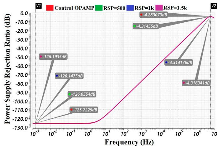
**Figure 8.** PSRR waveform behavior vs. frequency, with  $RS3 = RS4 = RSP$  (considered a parameter) and  $RS1 = RS2 = RSN = 0 \Omega$ .
