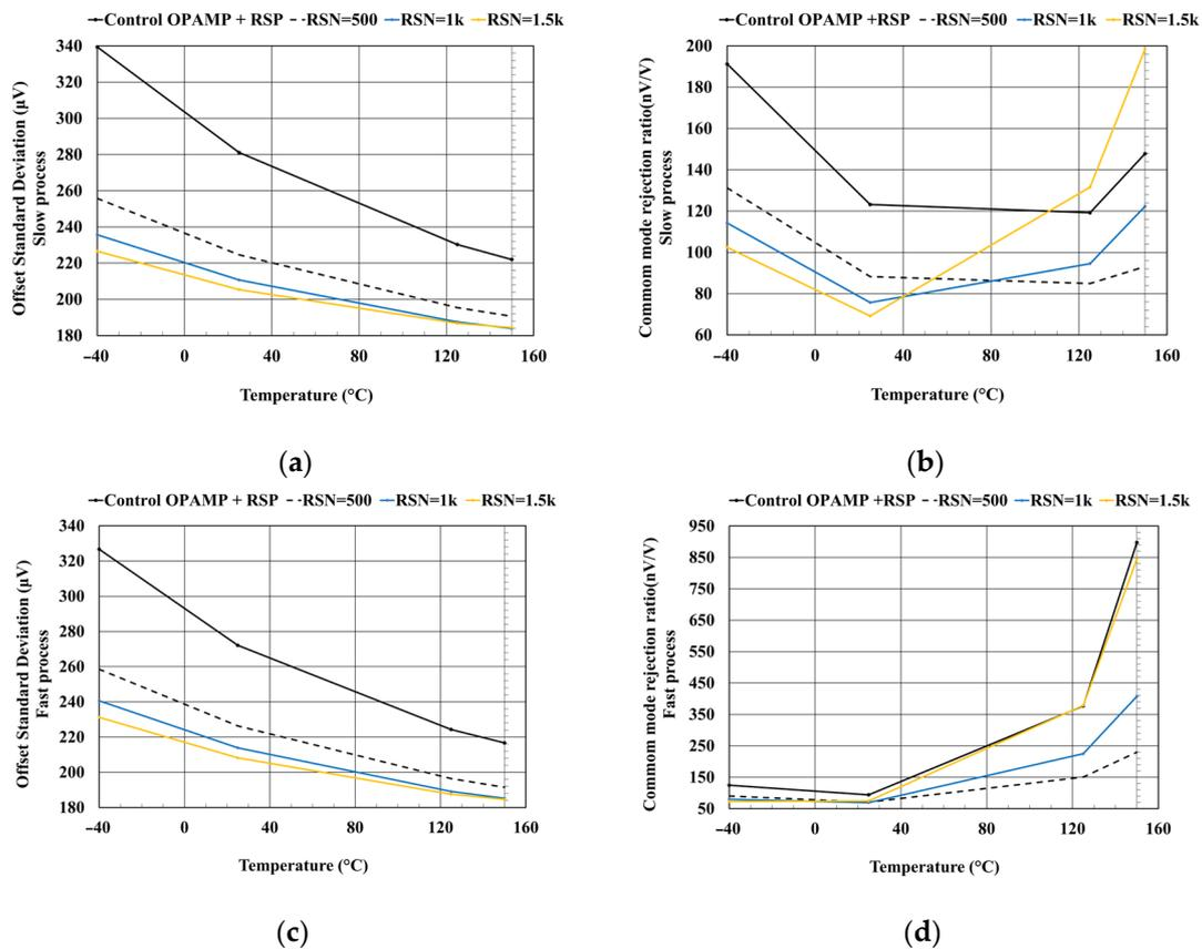
**Figure 13.** Process variation’s influence, with  $V_{DD} = 5 \text{ V}$ ,  $R_{S3} = R_{S4} = R_{SP} = 1 \text{ k}\Omega$ , and  $R_{S1} = R_{S2} = R_{SN}$  (considered a parameter). (a) Slow—offset voltage standard deviation distribution; (b) slow—CMRR standard deviation distribution; (c) fast—offset voltage standard deviation distribution; (d) fast—CMRR standard deviation distribution.
