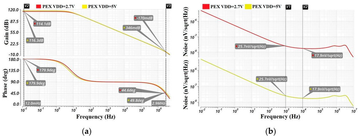
Figure 19. AC and noise performance after PEX. (a) Gain and phase waveforms; (b) voltage noise density.
