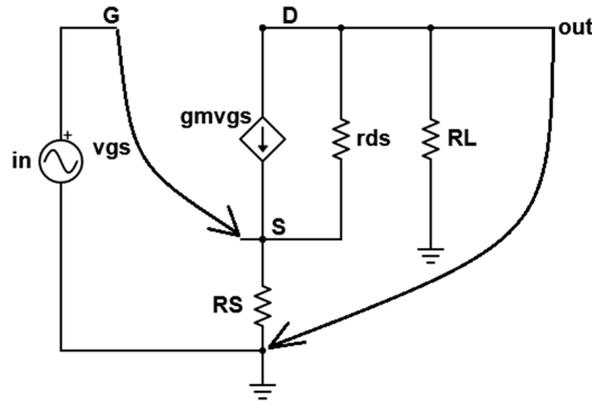
Figure 3. Small-signal schematic for common source with degeneration.
