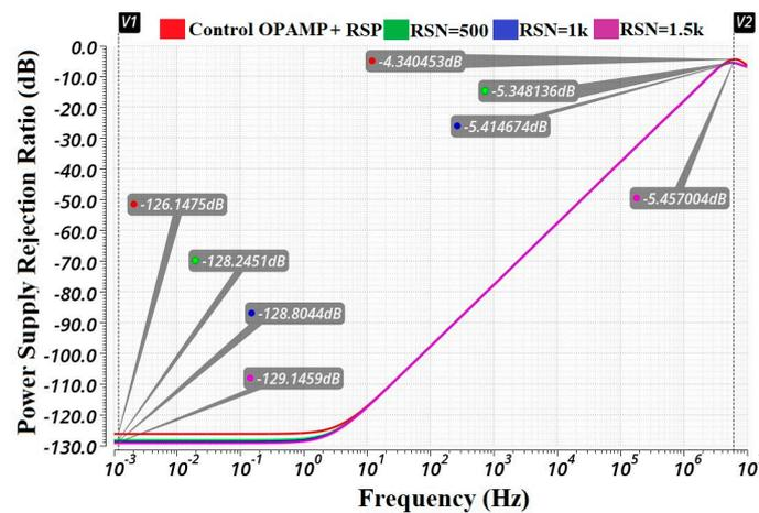
**Figure 14.** PSRR waveforms behavior vs. frequency, with  $R_{S3} = R_{S4} = R_{SP} = 1 \text{ k}\Omega$  and  $R_{S1} = R_{S2} = R_{SN}$  (considered parameters).
