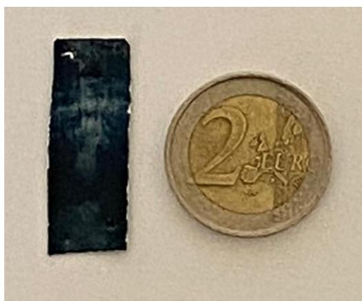
**Figure 3.** Fabricated bacterial cellulose device.
