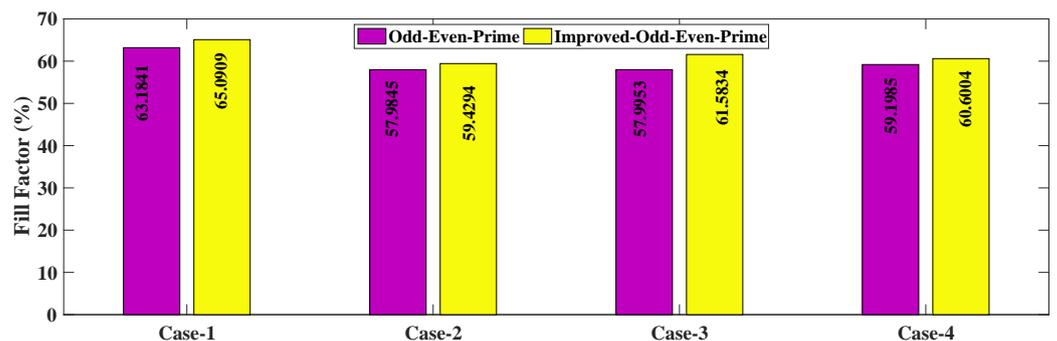
**Figure 13.** Fill-factor for  $9 \times 9$  PV array.
